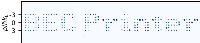
FIG. 6. Illustration of an experimental BEC dot-printer : each of the 67 columns of the image is an absorption image taken after a QOC preparation of an equal-weight superposition of momentum states chosen among \{|\chi_i\rangle, i \in \{-3, \dots, 3\}\} (see text).
