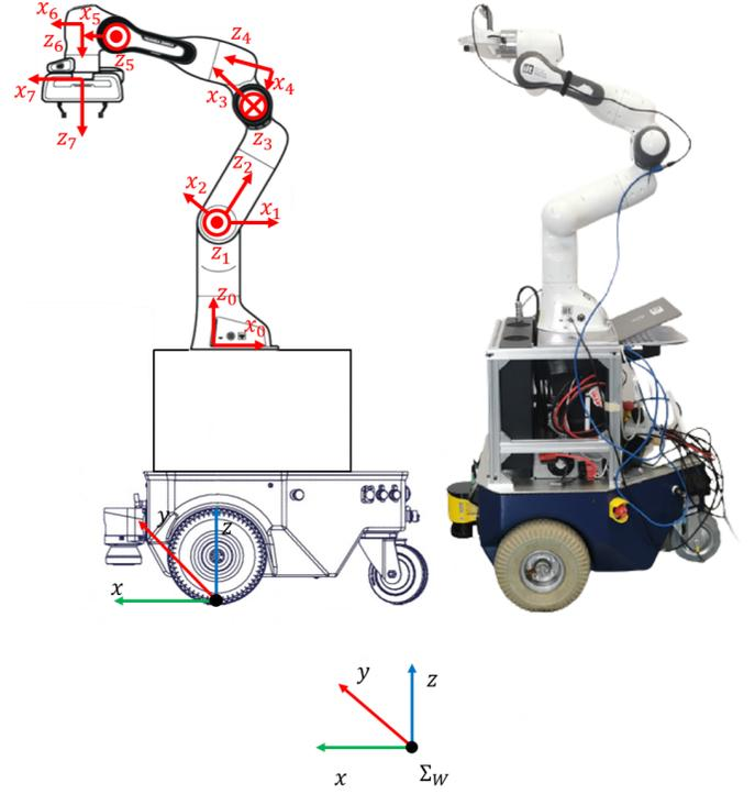
Fig. 3. Whole-body kinematic model of Rolling Panda
