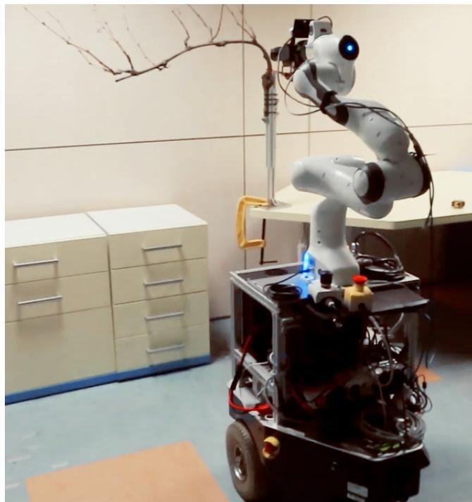
Fig. 1. An example of a robot grapevine pruning system Rolling Panda. To achieve this scenario, the following temporal sequences are followed: grapevine spur detection, whole-body motion to approach pruning point, and cutting the spur.
