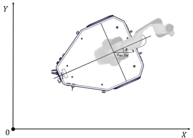
Fig. 2. Schematic drawing of Rolling Panda.  $x_m$ ,  $y_m$ , and  $\phi$  denote the center position and heading angle of the mobile platform with respect to the global coordinate.
