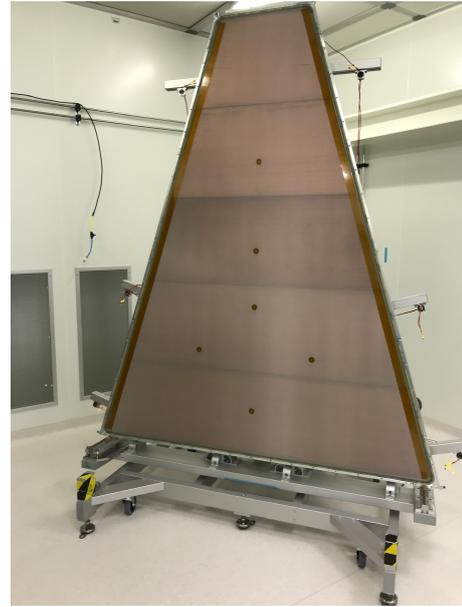
Figure 11: A drift panel fully equipped. The five drift PCBs with their copper cathode are distinguishable through the greyish mesh stretched on it.
