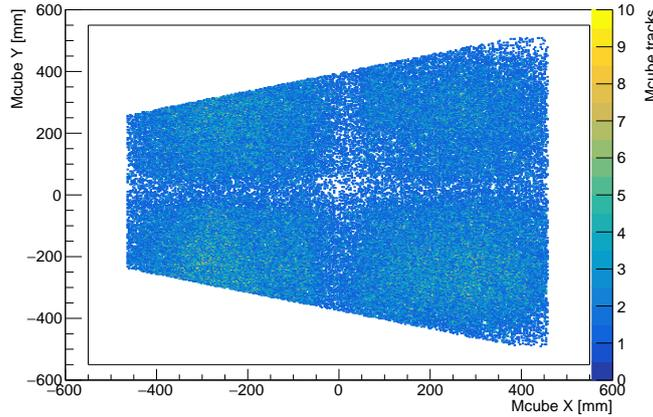
Figure 48: Distribution of  $M^3$  tracks extrapolated to the module plane on Layer 1. Number of  $M^3$  tracks during the data taking is binned per  $2.5\text{ mm} \times 2.5\text{ mm}$ . The acceptances of each bulk detector result in a cross with lower statistics. The outline of the  $M^3$  system is indicated by the solid lines.
