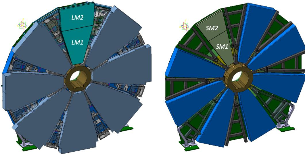
Figure 1: NSW detectors layout with the 8 large sectors (left) covering the 8 small sectors (right).
