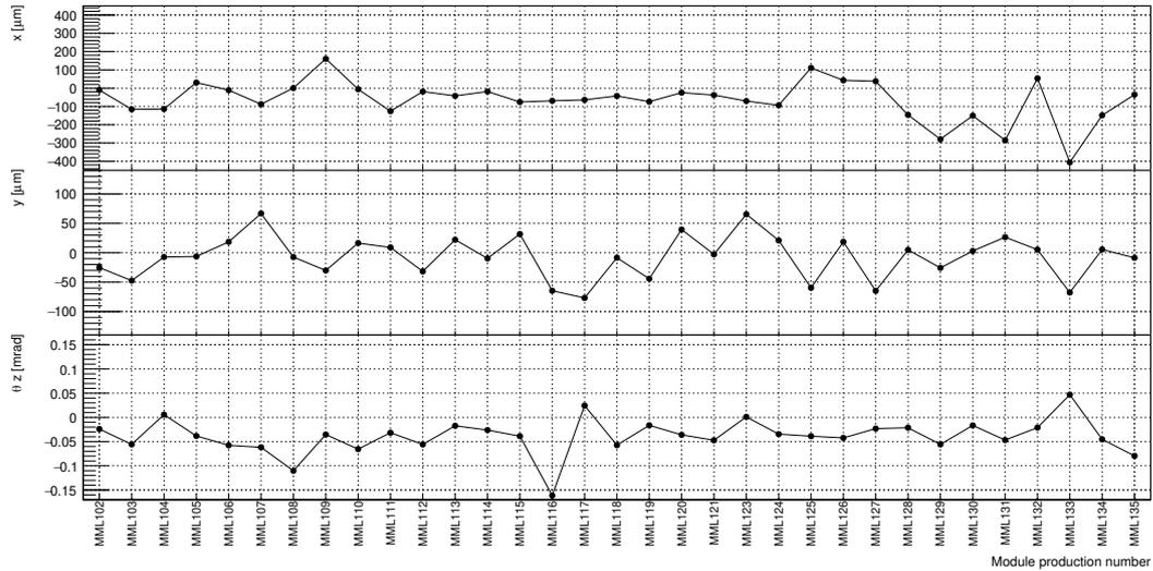
Figure 34: Metrology fit result: stereo panel position ( $x$  and  $y$ ) and rotation (about the  $z$  axis,  $\theta_z$ ) parameters, with respect to the eta panel, as a function of module production number. The parameters are expressed in the nominal frame of the stereo panel (which coincides with the nominal frame of the 5th PCB of the first layer, see Fig. 30).
