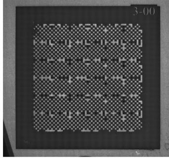
Figure 23: A Rasnik mask etched on PCB.
