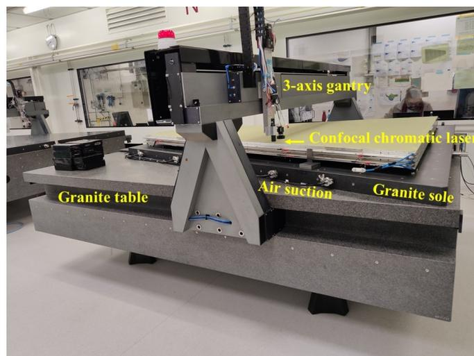
Figure 9: Planarity scan survey of a module.
