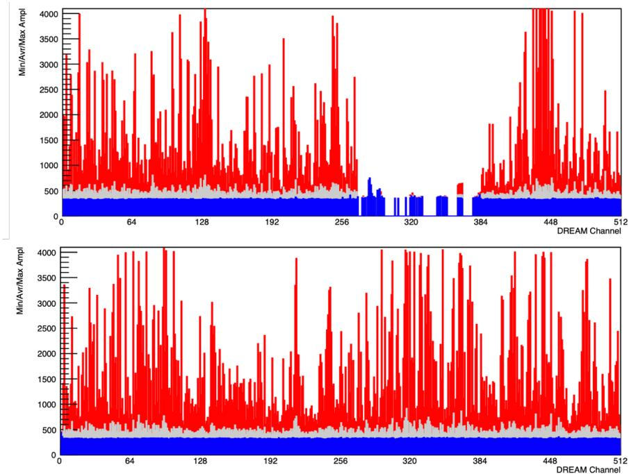
Figure 43: Hit maps for the 512 channels of one Front End Unit (same as Fig.42). The red, grey, and blue represent respectively the maximum, average, and lowest, values recorded over a one-hour run. The upper graph shows almost no signals on channels 256 to 354 due to a connection problem. The lower graph shows the same hitmap after re-fixing the connector to fix the issue.
