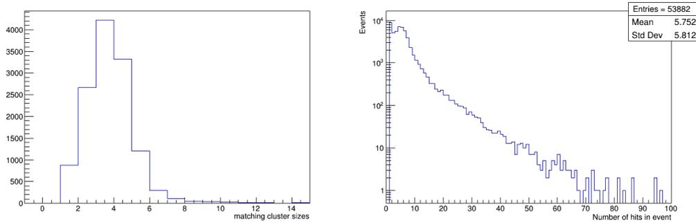
Figure 46: Left: Size of clusters matched to  $M^3$  tracks for the layer 1 of Module 11 PCB1. Right: Distribution of hit multiplicity in one FEU for events recorded in the module.
