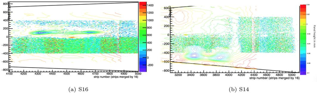
Figure 54: Comparison between signals observed on the cosmic test bench and the planarity scan made during construction. Contour lines correspond to height measurement from the planarity scans. The height is given by the vertical scales. The effect of holes is clearly seen in the inefficiency of detectors.
