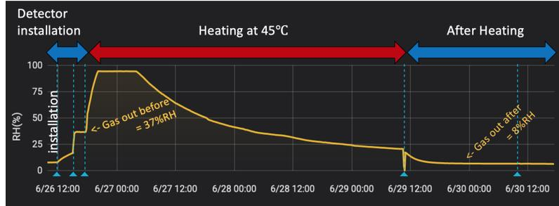
Figure 40: Gas relative humidity in % before and after the heating. Just after the connection of the module on the CTB gas system, the module output relative humidity is 37%. Then it is heated at 45 °C to help water out-gassing during three days. Once a stable mode is achieved (the humidity has decreased), the heating is turned off. The detector output reaches then 8% RH.
