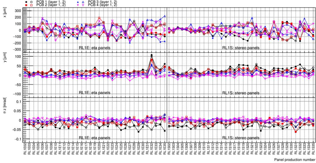
Figure 32: Metrology fit result: PCB position ( $x$  and  $y$ ) and rotation (about the  $z$  axis,  $\theta_z$ ) parameters, as a function of the panel production number. The different markers correspond to different PCB types and layers. The reported values are deviations of the different PCBs in their nominal frame (see Fig. 30). The layer frame is fixed on the 5th PCB, whose parameters are thus zero by definition, and are not reported in this plot.
