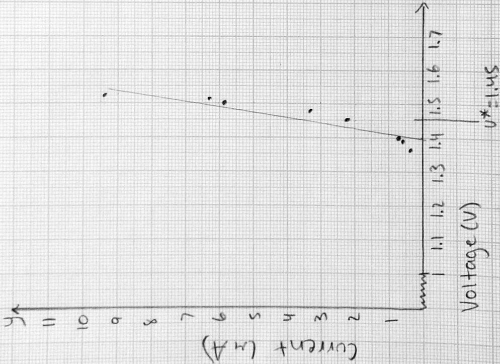
Current vs Voltage of LED 7
