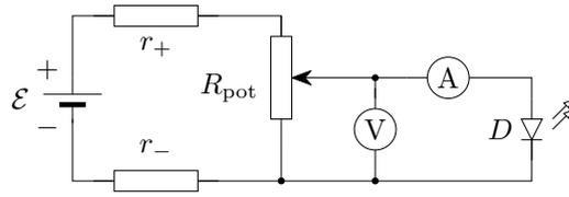
FIG. 10: Circuit for study current-voltage characteristics. Adjustable voltage regulator with potentiometer for voltage supplying to the LEDs and for investigation of  $I(U)$ . The voltage from the battery holder is applied to the potentiometer. The LED is connected to the middle terminal and to one of the other terminals of the potentiometer. The ammeter is connected in series with the LED and the voltmeter is connected in parallel.
