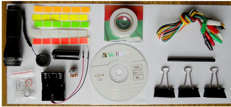
FIG. 1: Details of the set-up given to the participants: 1 small plastic bag containing 8 light emitting diodes (LED), 1 paper clip and 2 small rubber rings, 1 potentiometer, 1 piece of black plastic straw, 3 metal binder clips, 1 battery holder for 3 AA-type batteries, 1 double sided adhesive tape, 1 compact disk (CD), 7 connecting crocodile cables, 1 torch with battery holder taken out, 5 bands of 6 differently colored sticky labels.
