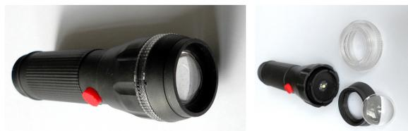
FIG. 7: Torch with lens: carefully unscrew the part holding the lens to the torch, disassemble it and take out the lens.
