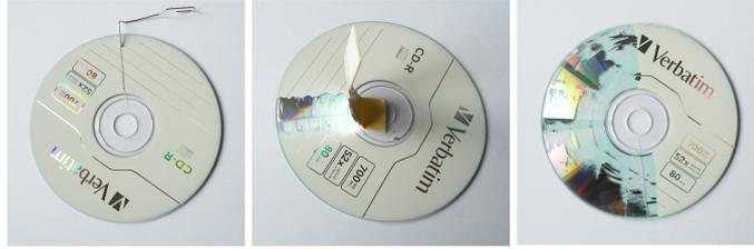
FIG. 6: The technology of peeling the foil of the compact disk: 1) The foil is scratched radially with the paper clip. 2) A piece of the adhesive tape is stuck on the scratch. 3) Then the piece is pulled and the foil stuck on the tape is removed from the CD. 4) Repeat steps 2) and 3) above (or near) the edges of the remaining foil until about half part of the disc is peeled from the foil as a half Moon at the right. You can use both sides of the double adhesive band.
