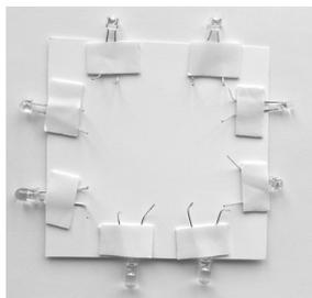
FIG. 5: Square piece with 8 LED stuck by double sided adhesive tape. Enumerate each LED and write a small (+) sign close to the number to mark the anode of LED. The terminals are bent in vertical direction in order to be bitten by crocodiles :-).
