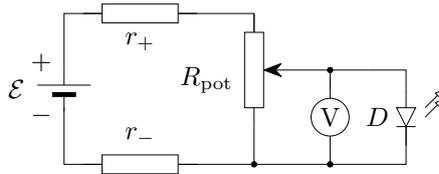
FIG. 4: LED connected to the voltage source from Fig. 3, circuit for measuring the voltage  $U^*$  at which the LED emits the weakest evanescent light.
