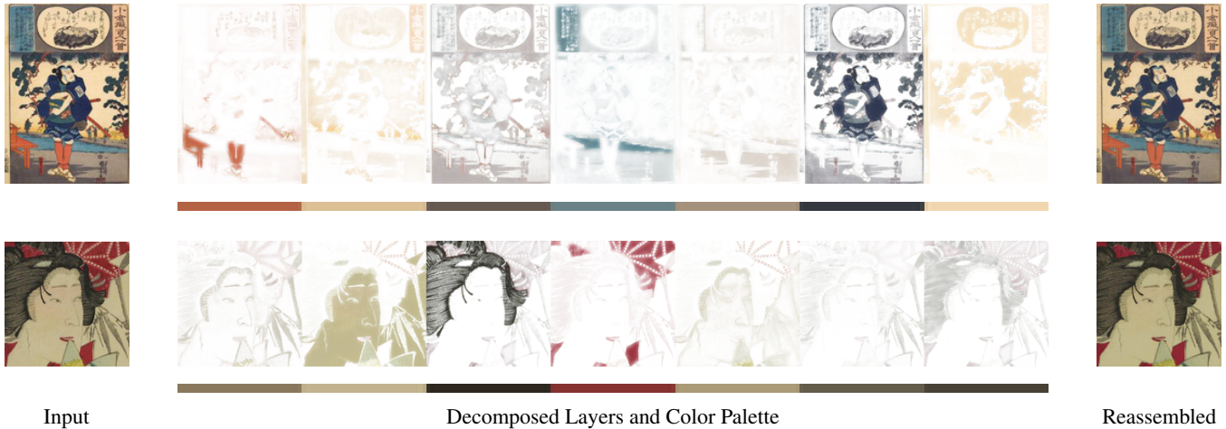
Figure 9: Soft color separation takes as input Ukiyo-e paintings (left) and a color palette (middle), and produces decomposed layers of homogeneous colors (middle). These layers can be used as the inferred woodblocks for corresponding colors and composed back to a reassembled painting (right) resembling the original one. We infer the color palette by applying K-means clustering (Lloyd 1982) on the input painting’s pixels.
