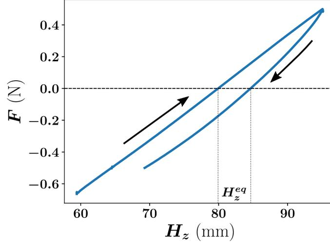
FIG. 9. Force-displacement response of the stack of 4 modules studied in section II B near the rest position for the configuration 0000. The dotted lines represent the limit values of  $H_z^{eq}$  we used in fig. 7
