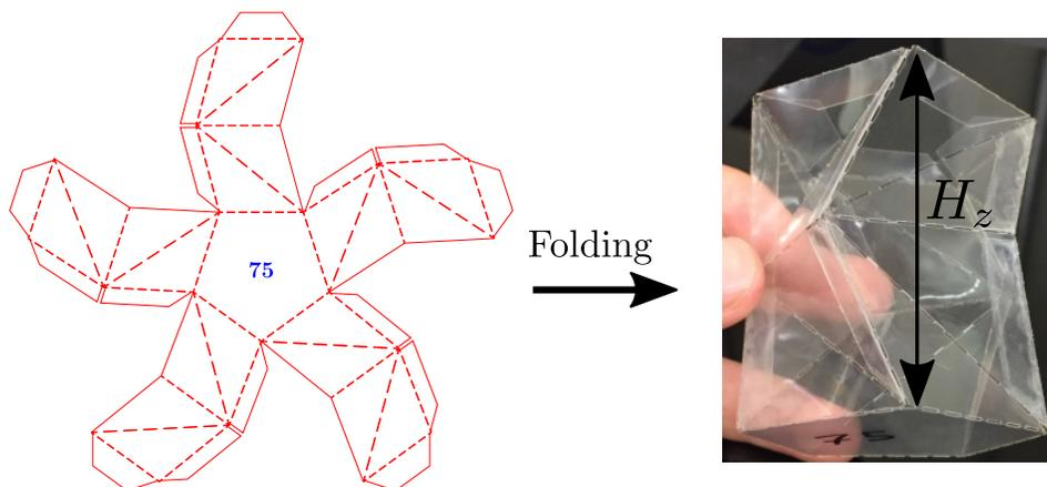
FIG. 2. Cutting pattern used to produce a single module with  $\ell_1 = 32$  mm,  $\phi_1 = 75^\circ$  and  $n = 5$  next to the resulting bellows after folding.  $H_z$  is the bellows' end-to-end height. The drawings are available online [42].
