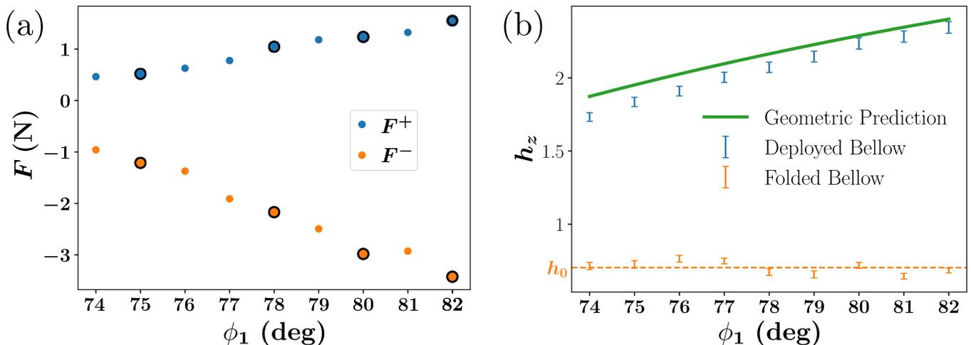
FIG. 4. (a) Force thresholds with respect to the pattern angle  $\phi_1$ . The four highlighted modules are those used in section II B. (b) Normalized height  $h_z = \frac{H_z}{\ell_1}$  measured for the folded and deployed configurations. The solid green line corresponds to the geometrical prediction of the deployed height given by eq. (3). The dashed orange line corresponds to the mean value  $h_0 = 0.70$  measured for the folded height.
