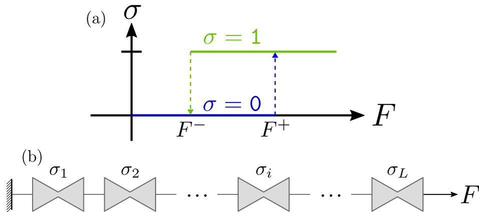
FIG. 5. Schematical description of the Preisach model. (a) Transition cycle for an hysteron  $\sigma$ , element with two stable configurations 1 and 0, with respect to the external loading  $F$ .  $F^+$  (resp.  $F^-$ ) is the loading threshold for the  $0 \rightarrow 1$  (resp.  $1 \rightarrow 0$ ) transition. (b) Stack of  $L$  independent hysterons  $\sigma_i$  in series symbolizing a stack of modules.
