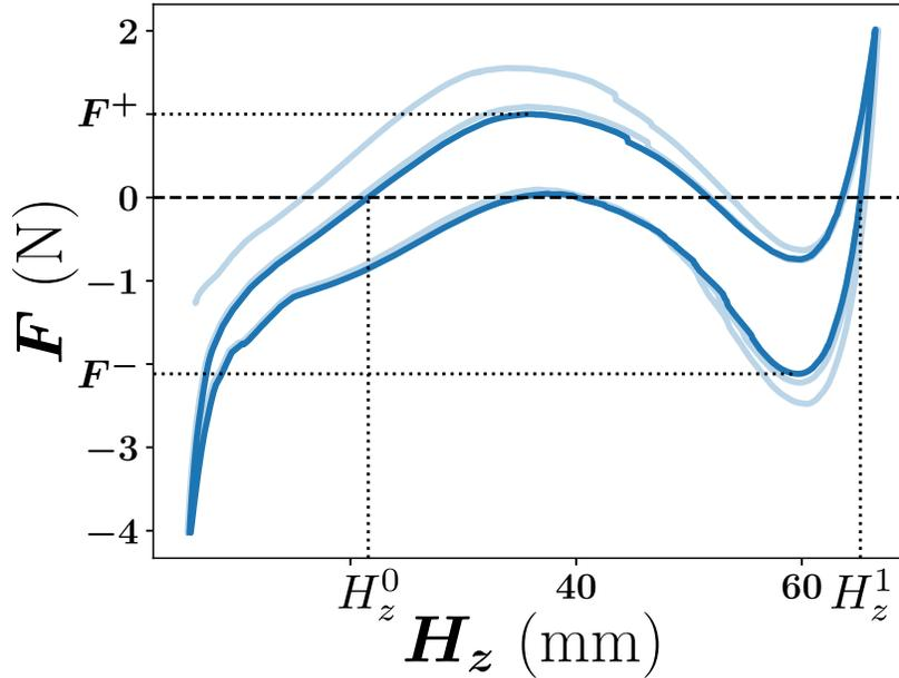
FIG. 3. Force-displacement response of a single module with  $n = 5$ ,  $\phi_1 = 78^\circ$  and  $\ell_1 = 32\text{mm}$  for 3 cycles of deployment-folding. The first two cycles are transparent while the last one is opaque.  $F^+ = 1.0\text{ N}$  and  $F^- = -2.11\text{ N}$  are the threshold forces between configurations. The heights for folded ( $H_z^0 = 21.6\text{ mm}$ ) and deployed ( $H_z^1 = 65.5\text{ mm}$ ) configuration are annotated.
