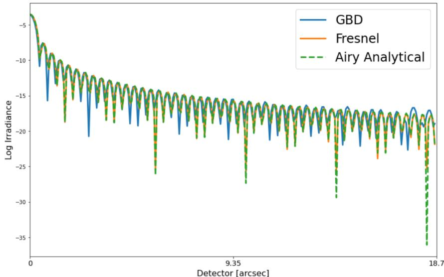
Figure 4. Cross-section of the focal plane intensity on a log scale generated by an ideal  $F/2.3$  lens using Gaussian Beamlets (blue) and Fresnel (orange) in comparison to the analytical airy function (green).
