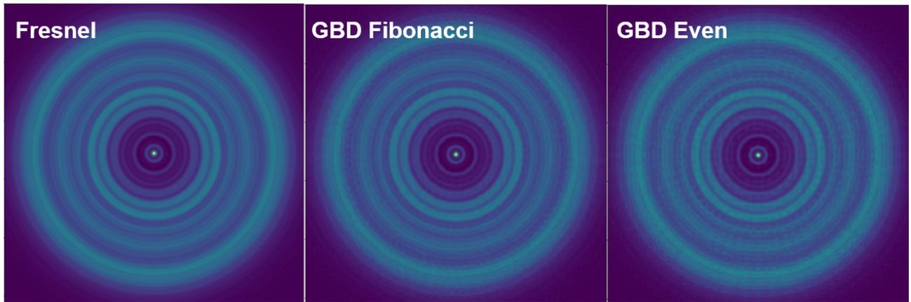
Figure 6. Comparison of Poisson's spot for cases of equal Fresnel number. (Left) POPPY's Fresnel propagator. (Middle) GBD propagator using Fibonacci sampling. (Right) GBD propagator using even sampling.
