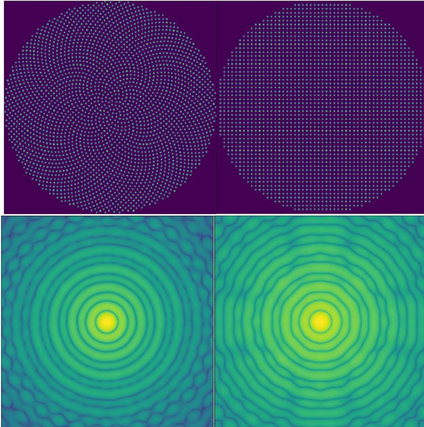
Figure 2. Demonstration of various sampling schemes (Right) Even sampling<sup>1</sup> (Left) Fibonacci sampling.<sup>11</sup> (Top) Undersampling in pupil plane to show beamlet distribution, (Bottom) The corresponding PSF.
