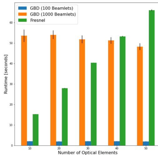
Figure 8. Comparison of runtime between GBD POPPY’s Fresnel mode for increasing number of optical elements. Due to GBD’s reliance on raytracing for propagation, the runtime is dominated by the number of beamlets used rather than the number of elements, making it ideal for many-element systems.
