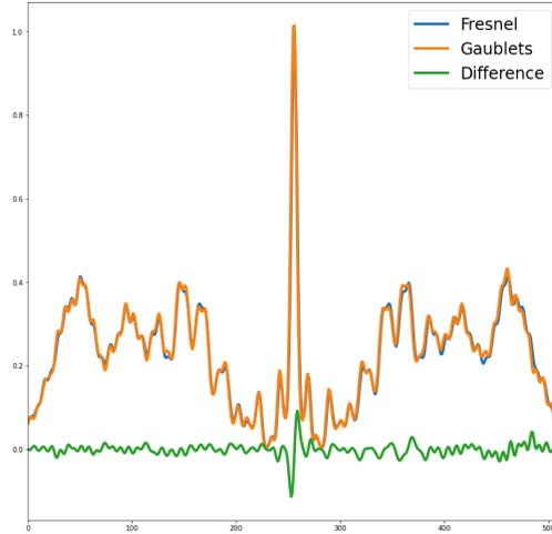
Figure 7. Cross-section of the Fresnel and GBD Fibonacci results from Fig 6 superimposed with the difference of the Fresnel distribution with the GBD distribution.
