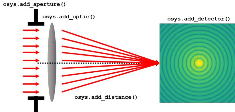
Figure 3. (Top) Sample code to demonstrate the user-friendly & object oriented construction of the GBD module and (Bottom) a graphical representation of what the code creates.
