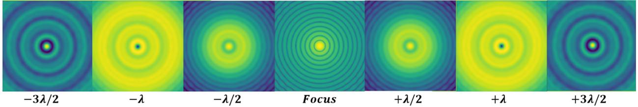
Figure 5. Field intensity distribution near the focal plane at  $n\lambda/2$  waves of defocus. The on-axis irradiance is expected to maximize at half-integer waves of defocus and minimize at integer waves of defocus. Recovering this result using GBD is proof that the method is capable of accurately modeling intensity distributions near the focal plane.
