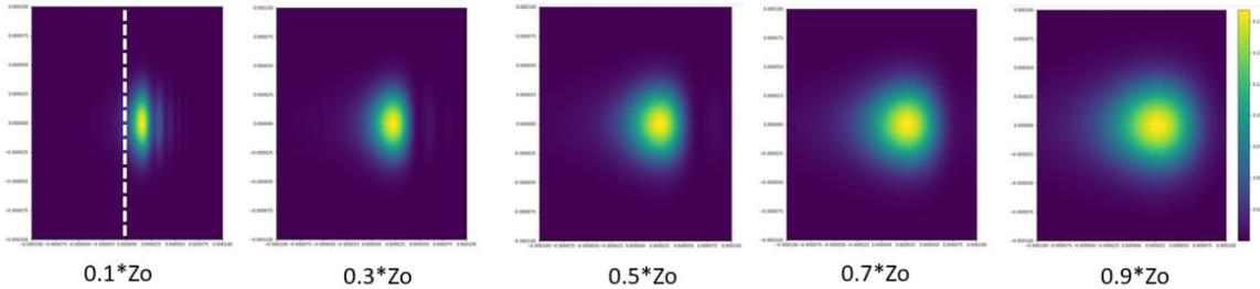
Figure 9. Propagation of a half-truncated Gaussian beam at fractions of the Rayleigh range. Observed here are the near-field diffraction effects that result from capturing higher spatial frequency information at a hard aperture (white dashed line).
