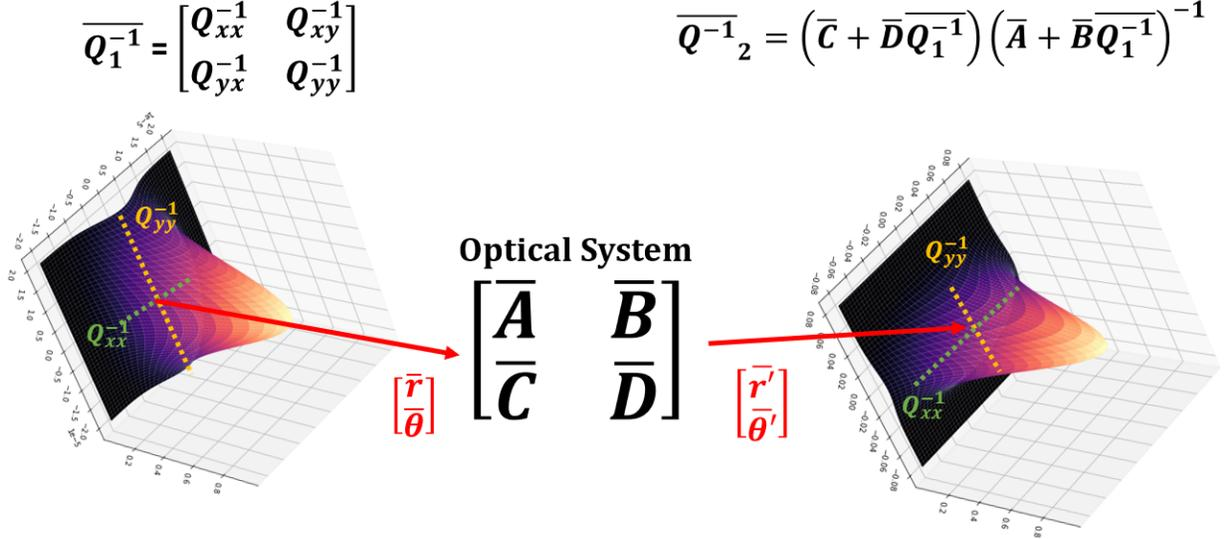
Figure 1. Gaussian beamlets are defined by a paraxial "central ray" (shown in red) that locates the Gaussian beam, and a complex curvature matrix that tracks the waist radius and curvature ( $\overline{Q}_1^{-1}$ ). Utilizing the linear laws of paraxial ray tracing, physical optics phenomena can be modeled.
