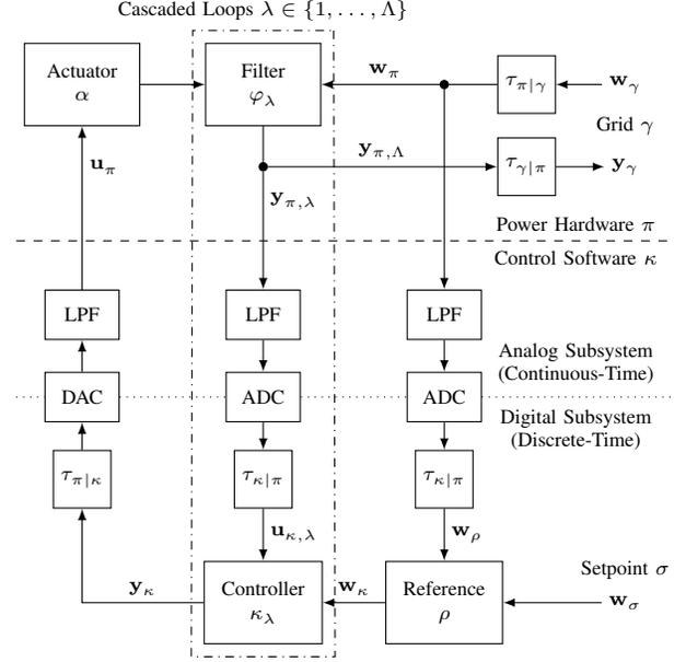
Fig. 2. Schematic diagram of a generic CIDER. The power hardware  $\pi$  consists of the actuator  $\alpha$  and cascaded filters  $\varphi_\lambda$  (for simplicity, one stage is shown only), the outermost of which is connected to the grid  $\gamma$ . The control software  $\kappa$  consists of the reference calculation  $\rho$  and cascaded controllers  $\kappa_\lambda$ , which track the setpoint  $\sigma$ . The transforms  $\tau$  represent changes of electrical connection or reference frame.
