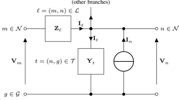
Fig. 1. The grid is represented by branch elements with compound impedance  $\mathbf{Z}_\ell$  and shunt elements with compound admittance  $\mathbf{Y}_t$ .  $\mathbf{I}_\ell$  and  $\mathbf{I}_t$  are the current flows through the branch and shunt elements, respectively.  $\mathbf{V}_n$  and  $\mathbf{I}_n$  are the phase-to-ground voltages and injected currents, respectively.
