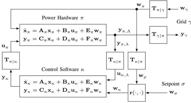
Fig. 3. Block diagram of the proposed generic state-space model of CIDERs. Note the modularity: power hardware  $\pi$ , control software  $\kappa$ , and grid  $\gamma$  are represented by separate blocks, which are interfaced via coordinate transformations. The reference calculation  $\mathbf{r}(\cdot, \cdot)$  may be either linear (i.e., for  $Vf$  control) or nonlinear (i.e., for  $PQ$  control). The other blocks of the model are exactly linear (i.e., LTP systems and LTP transforms).
