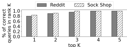
Figure 5. Cumulative distribution (per app) of the rank of the correct query over our test set of repeat faults.
