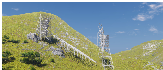
Fig. 16: BINGO concept view. The optics alignment follows a north-south line, with the primary reflector pointing north. The control cabin is fully isolated electromagnetically and it is located behind the hill on the left.
