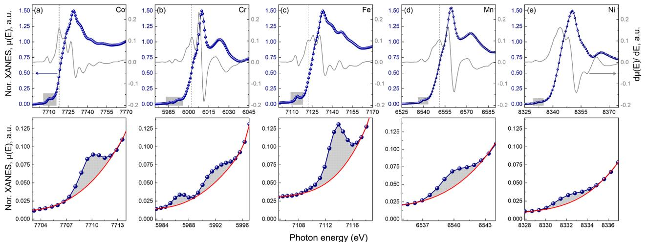
Figure 4. The XANES spectra,  $\mu(E)$  (blue), the first order derivative,  $d\mu(E)/dE$  (grey) and the integrated intensity of the pre-edge region (bottom) at the TM  $K$ -edges of S-HEO. Cr, Mn and Ni exclusively occupy the  $O^H$  sites, Co occupies the  $T^D$  site and Fe occupies both with predominant  $T^D$  occupancy.
