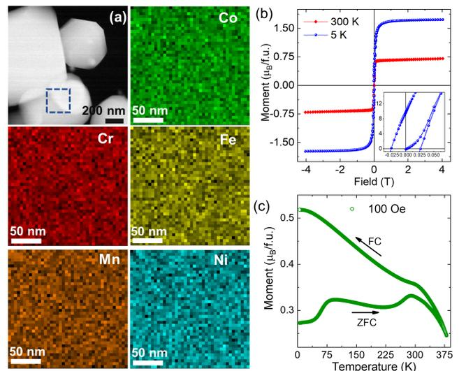
Figure 2. (a) Scanning TEM micrograph and the corresponding elemental distribution maps for Co, Cr, Fe, Mn and Ni. (b) M-H plots of S-HEO at 300 K and 5 K with the inset showing the virgin curve measurement at 5 K. (c) ZFC-FC data in the M-T plot at 100 Oe indicate a series of magnetic transition in S-HEO with the ferrimagnetic transitions occurring above 380 K.
