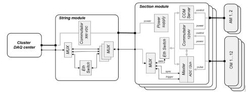
Figure 1. Block diagram of the experimental string.
