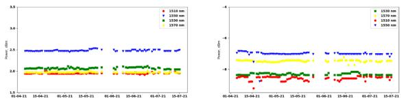
**Figure 2.** Time dependence of the power of the transmitters (left) and receivers (right) of optical transceivers for one section.
