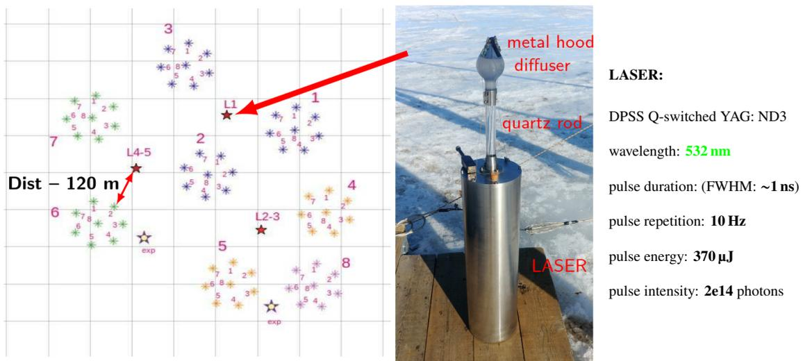
**Figure 1:** Left: Clusters map for 2021. The positions of the lasers (L1-L5) are marked by red stars. Strings with lasers are placed about 120 m from the nearest instrumented string. Right: Laser in a pressure housing, equipped with a lightguide and a diffuser with a metal hood (reflector) on the top.
