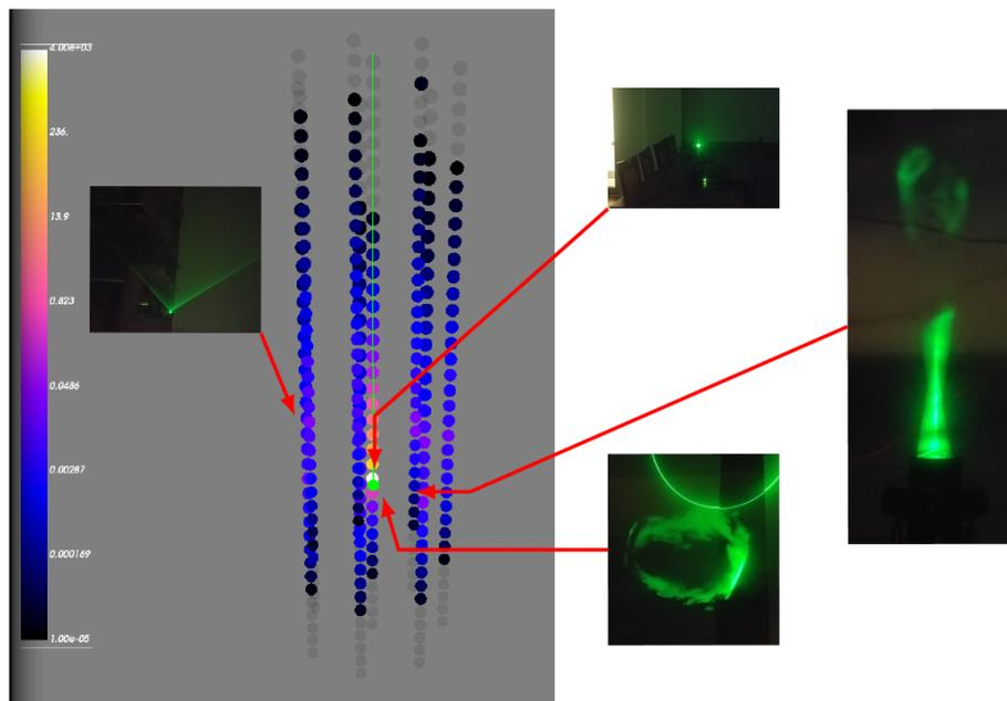
**Figure 6:** Simulation result for the laser attached to the center string of a cluster, equipped with Axicon (20°), for upgoing beam in water. The pictures on the right shows the real view of the laser beam, shaped into a cone in water mist (65 %RH), seen from the indicated points of the simulated cluster.
