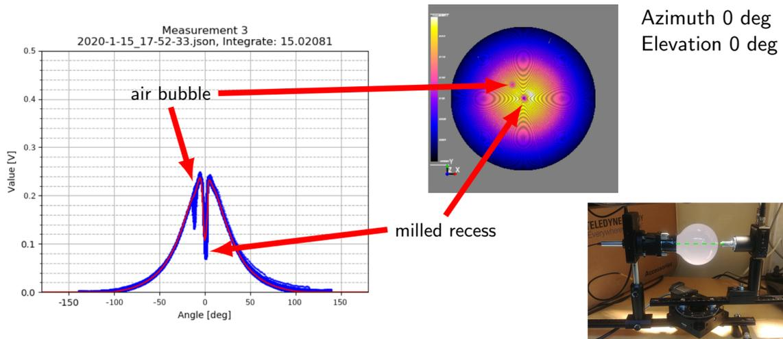
**Figure 3:** Near scan result. The plot shows averaged measurements from many planes. On the right side the 3D visualization showing the upper part of the diffuser. On the picture below, the configuration of the test bench for near scan. The dashed green line represents the Z axis, perpendicular to the picture above.
