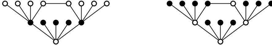
(a) Optimal  $(1, 2)$ -Color solution covering 13 edges. (b) Maximum independent set of size 10.
