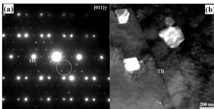
Figure 6. TEM characterization on TB (twin boundary): (a) SADP recorded on  $[011]$  zone axis and (b) Dark field image corresponds to the precipitate reflections inside the circle in Figure 6a.
