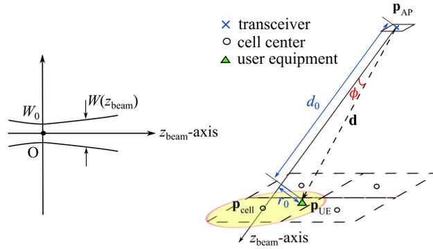
Fig. 2: Geometrical representation of the elliptical Gaussian beam.
