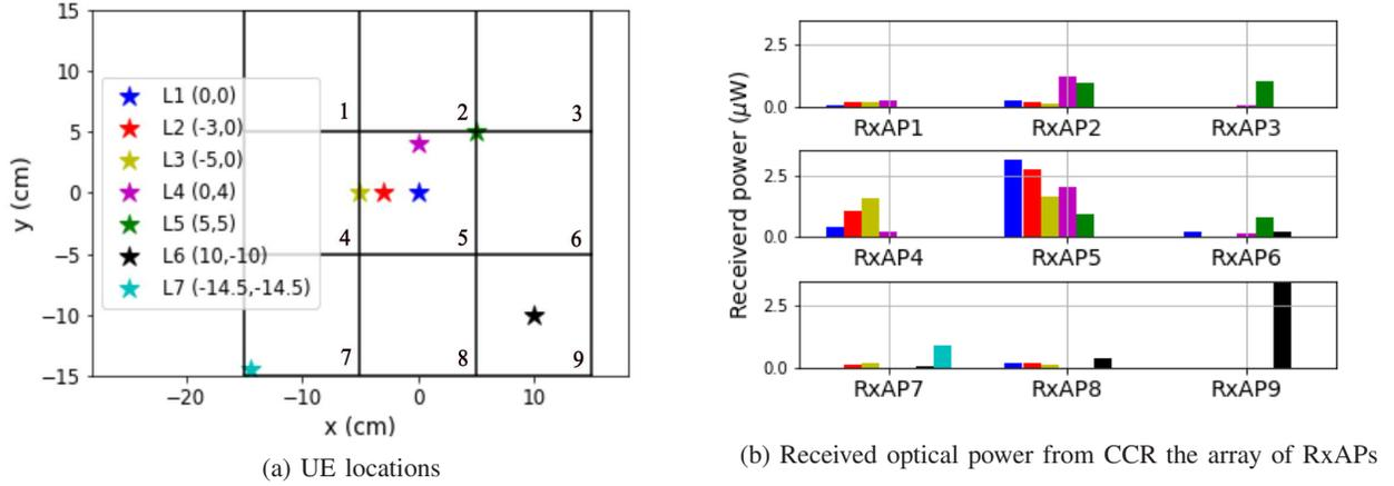
Fig. 8: The UE locations and received power matrix,  $N_{\text{beam}} = 9$ .
