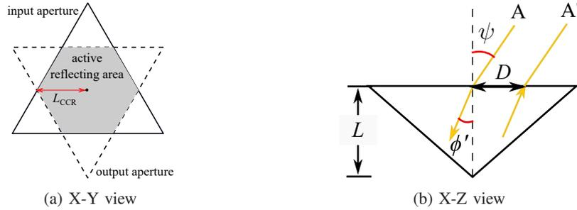
Fig. 3: Corner-Cube retroreflector
