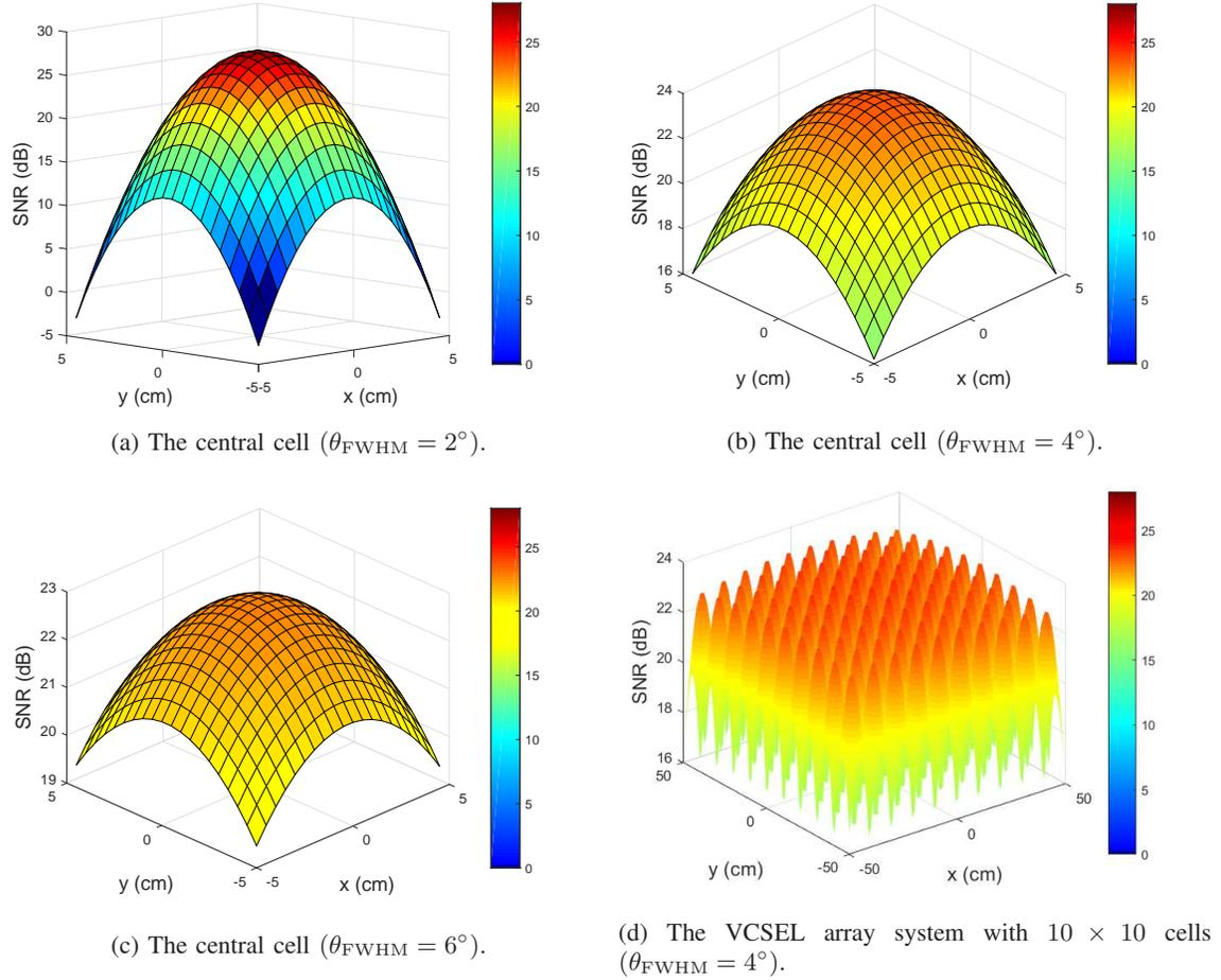
Fig. 10: SNR distribution in a single user system.
