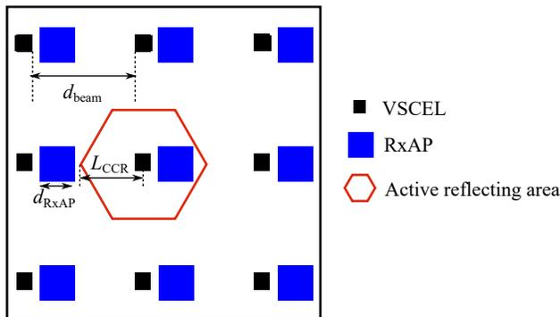
Fig. 4: The setup of the AP in the VCSEL array system using a CCR ( $N_{\text{beam}} = 9$ ).
