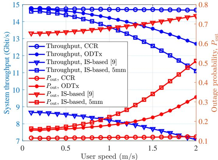
Fig. 14: Evaluation of system throughput and outage probability corresponding to user speed. ( $N_{\text{beam}} = 10 \times 10$ ,  $d_{\text{cell}} = 10$  cm,  $\theta_{\text{FWHM}} = 4^\circ$ ),  $N_{\text{UE}} = 5$ .
