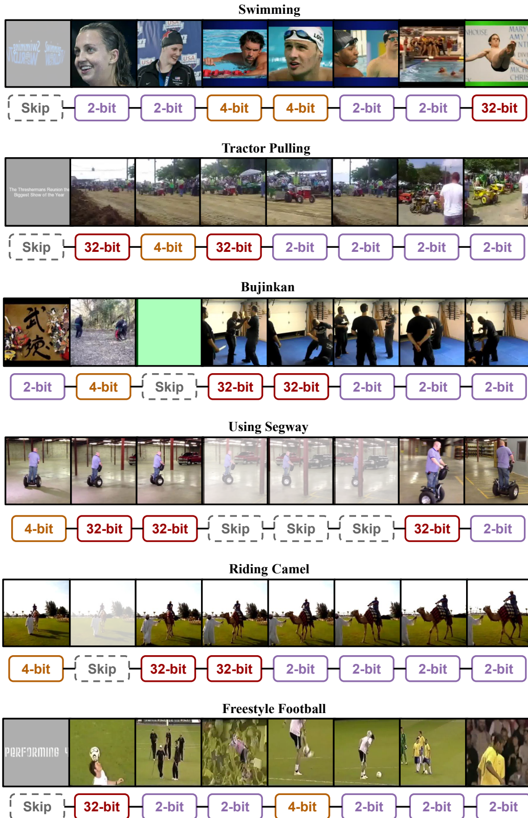
Figure 6: Qualitative examples. Our proposed approach VideoIQ processes more informative frames with high precision and less informative ones with lower precision or skip them when irrelevant, for efficient video recognition. Best viewed in color.
