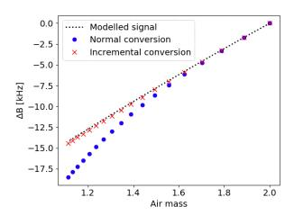
**Fig. 3.** Background response,  $\Delta B$ , as a function of air mass, am, for the skydip model. In black: modeled input data. In blue: calculated data with normal conversion method. In red: calculated data with "incremental method". The signal is negative because the tuning is at high air mass (am=2) and the background signal diminishes at lower am.
