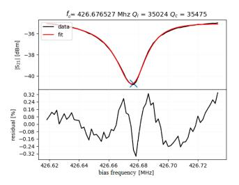
**Fig. A.1.** Amplitude signal,  $|S_{21}(f)|$ , as a function of the bias frequency, f. The resonance curve is fitted to characterize the pixel. Top: Single pixel bias signal (in black) and fitting Eq. A.3 (in red). The blue cross identifies the resonance frequency. Bottom: Percentage residual of a good fit between data and model.
