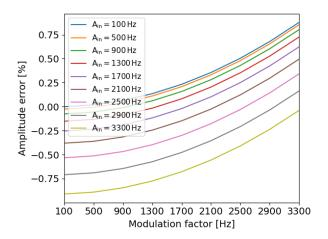
**Fig. 5.** Systematic error in percentage variation of the interferogram amplitude as a function of modulation factor,  $\Delta f_{\rm LO}$ . The background is fixed at 0 Hz. The error on the calculation converges to 0 % when the modulation factor approaches  $A_{\rm in}$ .
