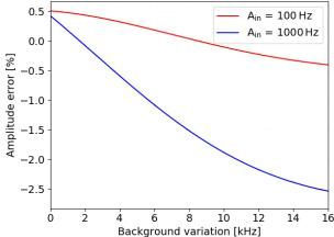
**Fig. 4.** Left: Conversion factor, *C*, variation as a function of background variation. Right: Bias in percentage in the reconstruction of the interferogram amplitude, *A*, as a function of background variation. The modulation factor is fixed at 2.5 kHz.
