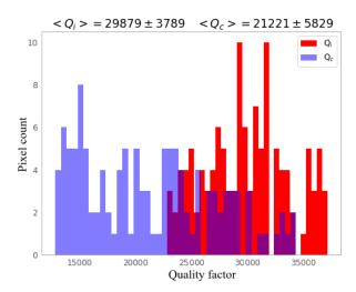
**Fig. A.2.** Quality-factor histograms measured on the A KISS array (for the best  $\sim 30$  % pixels). The  $Q_{\rm i}$  measured with a flat-field background of 50 K that models the sky is shown in red and  $Q_{\rm c}$  is shown in blue. The quality factors are represented in shadowed colors. The pixels are well distributed around suitable values, and the scatter is due to the different pixel designs that vary the resonance frequency and to slight fabrication defects.
