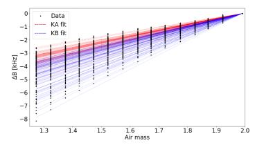
Fig. 6. Background response,  $\Delta B$ , as a function of air mass. One example skydip for the best ~42% of the pixels, selected by a Chi-squared test. Black dots: binned signal. Red/blue dashed line: skydip fit distinguished per array. The signal is negative because the tuning is at high air mass (am=2) and the background signal diminishes at lower am.
