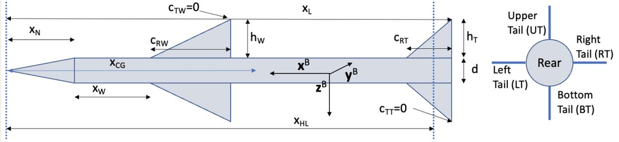
**Fig. 6 Missile Geometry**
