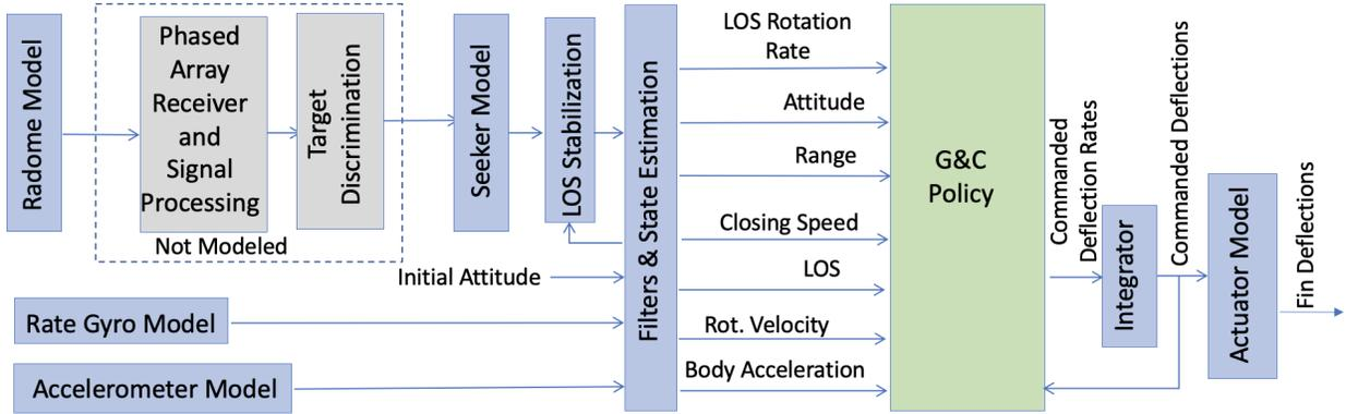
Fig. 1 System Diagram of GN&C system
