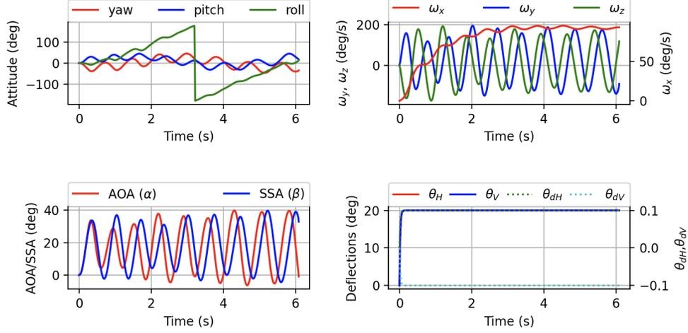
**Fig. 9 Open Loop Airframe Response to Fin Deflection, Altitude = 15 km**
