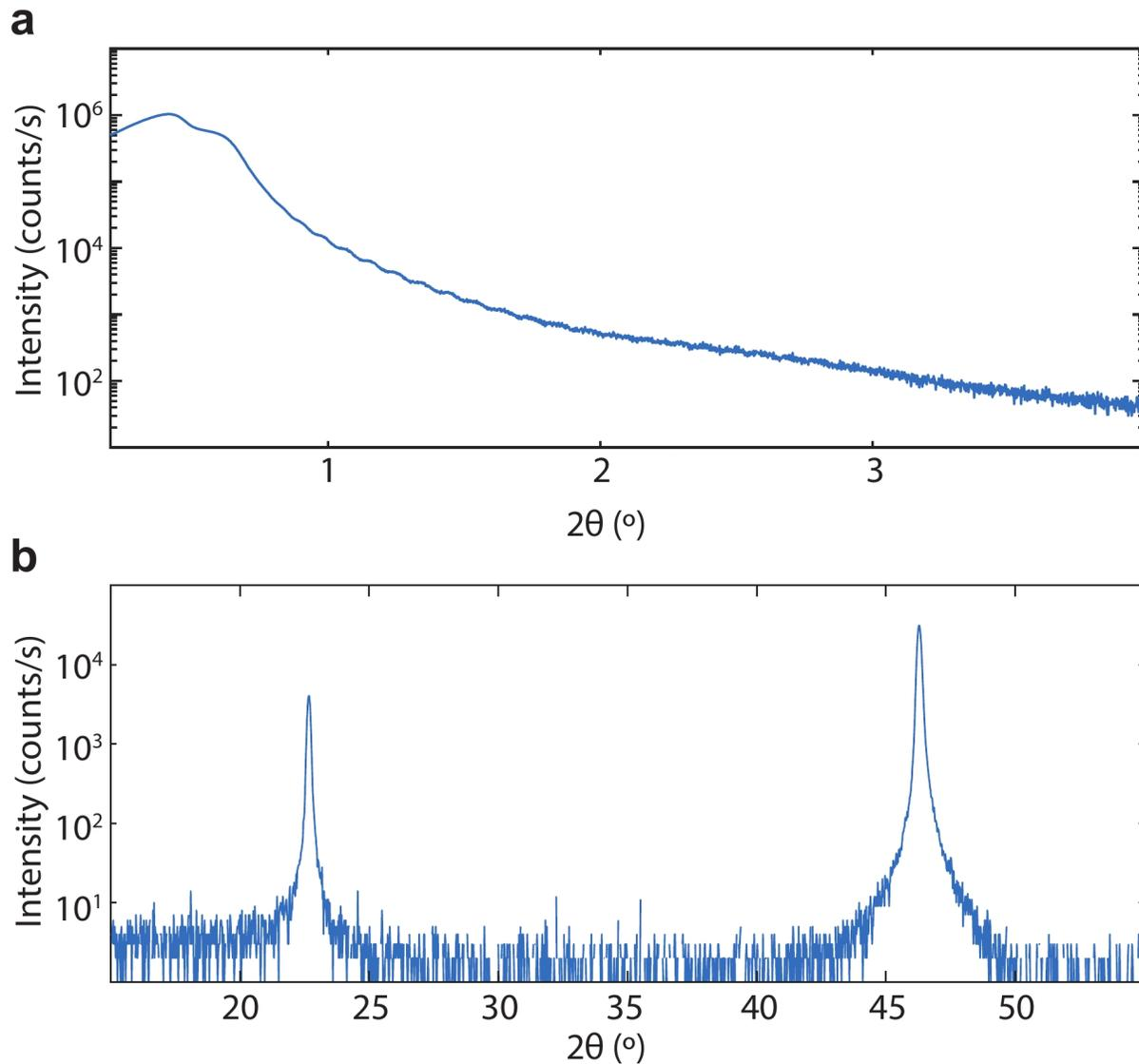
FIG. S2. **a** X-ray refractometry (XRR) performed on free-standing STO stamped on SiO<sub>2</sub>/Si. **b** X-ray diffraction (XRD) of the same film showing STO (001) and STO (002) peaks.
