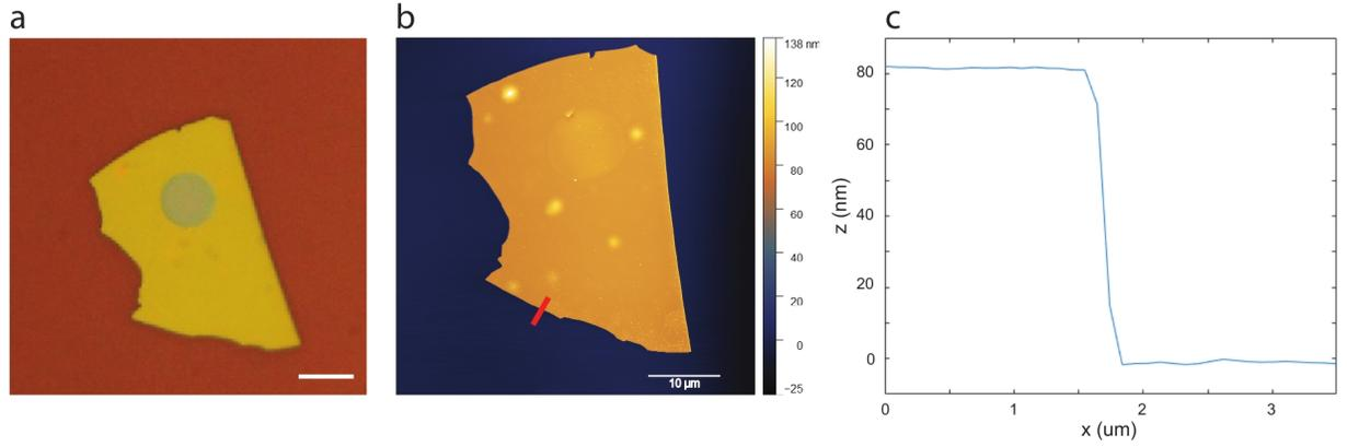
FIG. S3. **a** Optical image of a STO flake suspended over a 10  $\mu\text{m}$  cavity. Scalebar: 10  $\mu\text{m}$ . **b** Atomic force microscopy (AFM) image of the device. Red line indicates where a profile is taken. **c** Profile at the edge of the flake as indicated by the red line in **b**. Thickness of 82 nm is measured.
