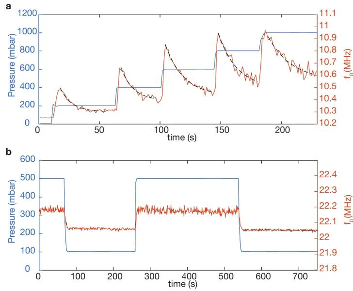
FIG. S5. Pressure (left y-axis, blue) response of mechanical resonance (right y-axis, orange) of STO **a** before annealing **b** and after annealing. Black dashed lines are the decay curves taken to extract the permeation time constant  $\tau_p$ .
