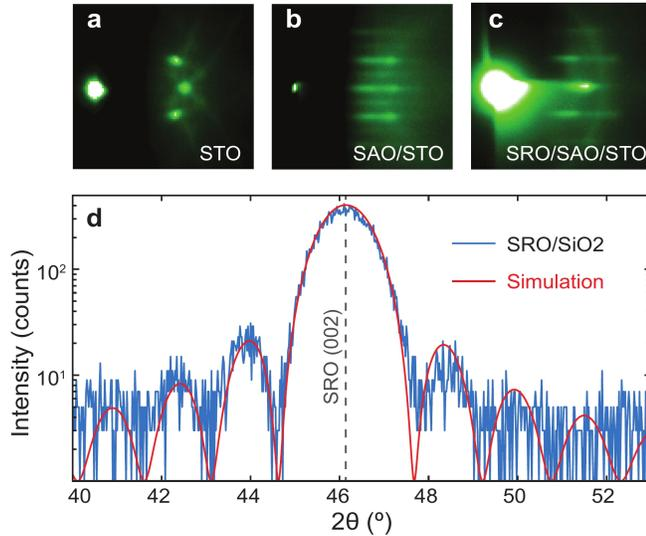
FIG. 1. Reflection high energy electron diffraction (RHEED) images of **a** SrTiO<sub>3</sub> (STO) substrate, **b** Sr<sub>3</sub>Al<sub>2</sub>O<sub>6</sub> (SAO) grown on STO substrate and **c** SrRuO<sub>3</sub> grown on SAO/STO stack. **d** X-Ray diffraction (blue) of exfoliated SRO stamped on SiO<sub>2</sub>/Si and the simulation (red). The c-axis lattice parameter extracted from the simulation is 3.931 Å and the thickness is 16 unit cells.
