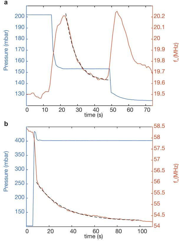
FIG. S6. Pressure response (left y-axis, blue) of mechanical resonance (right y-axis, orange) in a SRO device fabricated on 350 nm  $\text{Si}_3\text{N}_4/\text{Si}$  **a** before annealing, and **b** after annealing. Dashed black lines are exponential fits to extract the  $\tau_p$ . Before annealing,  $\tau_p = 6.02$  s and after annealing  $\tau_p = 22.5$  s.
