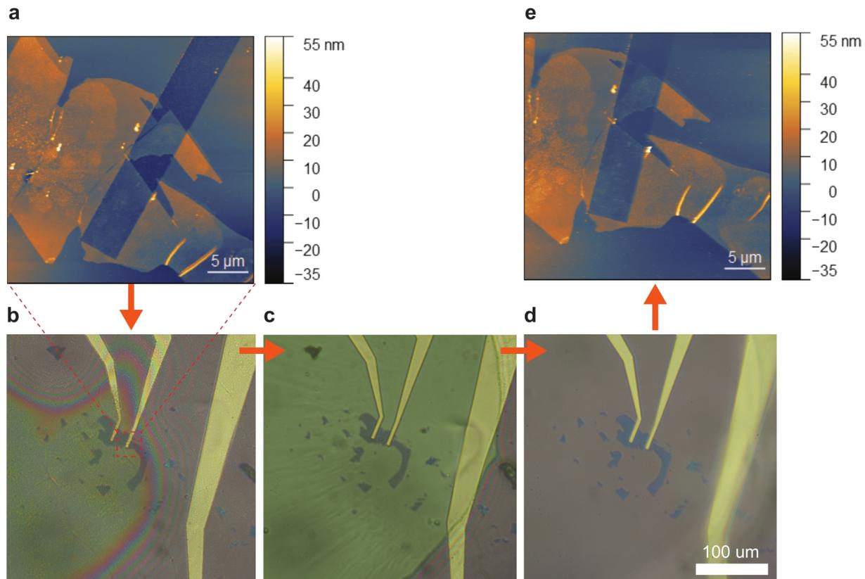
FIG. S10. AFM and optical microscopy images highlighting the inability to pick up the flakes of annealed SRO on  $\text{SiO}_2/\text{Si}$ . Polycarbonate is used as a sticky polymer to transfer the flakes. **a** AFM image of an annealed flake on top of a recessed electrode. **b-d** Optical images of the attempt to pick up the annealed flake using polycarbonate/ PDMS. **e** AFM image of the same same area after the pickup attempt.
