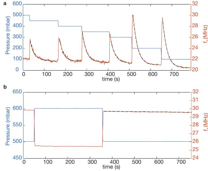
FIG. S4. Pressure (left y-axis, blue) response of mechanical resonance (right y-axis, orange) of SRO **a** before annealing **b** and after annealing. Black dashed lines are the decay curves taken to extract the permeation time constant  $\tau_p$ .
