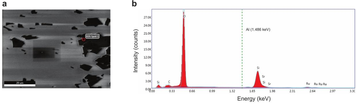
FIG. S7. **a** Scanning electron microscopy image of free-standing SRO stamped on SiO<sub>2</sub>/Si taken at 52 degree tilt . The spot where energy dispersive X-ray spectroscopy (EDX) is performed is indicated with a marker. **b** EDX of the film showing contributions from Si, O, Sr and Ru but not Al (1.486 keV green dashed line) suggesting that Sr<sub>3</sub>Al<sub>2</sub>O<sub>6</sub> is fully etched away in water.
