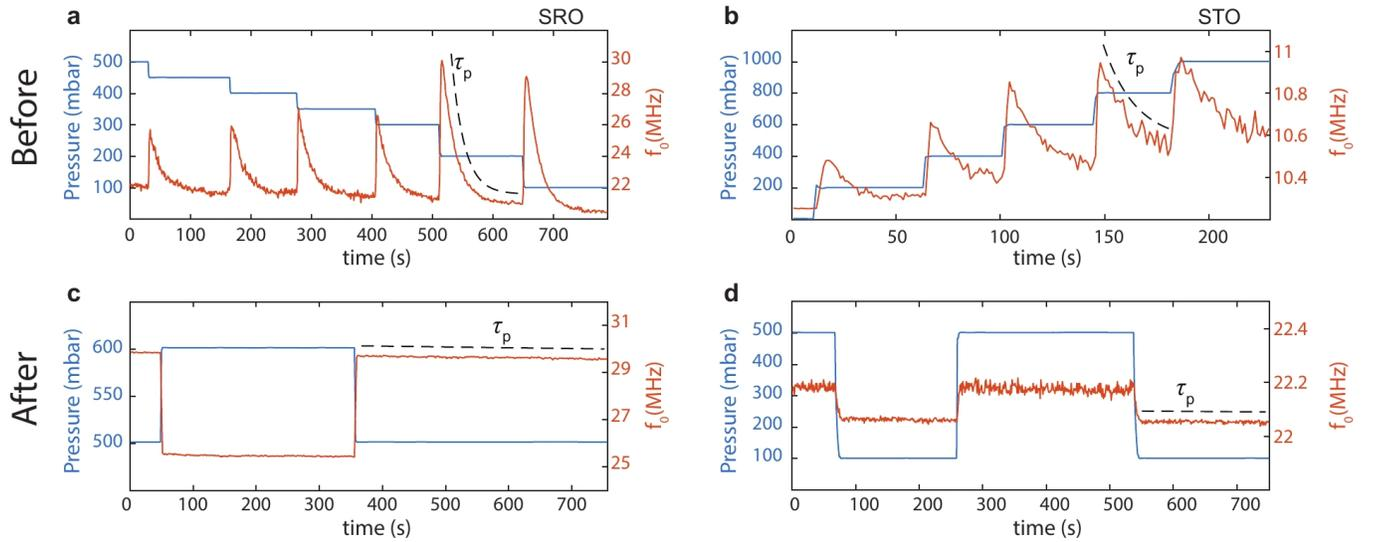
FIG. 3. Pressure response of the resonance frequency before (**a**&**b**) and after (**c**&**d**) annealing. Left column shows the behavior of a 16 unit cell (6.3 nm) SRO device and the right column shows the behavior of 82 nm STO device. The external pressure controlled by the pressure controller is plotted in blue on the left y-axes and the resonance frequency is plotted in orange on the right y-axes.
