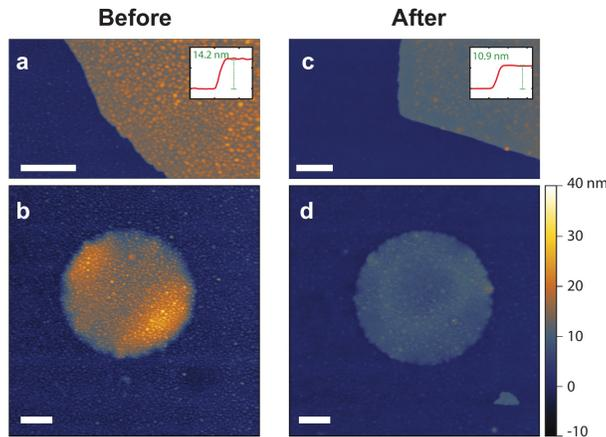
FIG. S11. **a** Atomic force microscopy (AFM) image of the edge of the SRO flake before annealing. The inset shows the step height of 14.2 nm. **b** AFM image of the suspended drum before annealing. **c** AFM image of the edge of the SRO flake after annealing. The inset shows the step height of 10.9 nm. **d** AFM image of the suspended drum after annealing.
