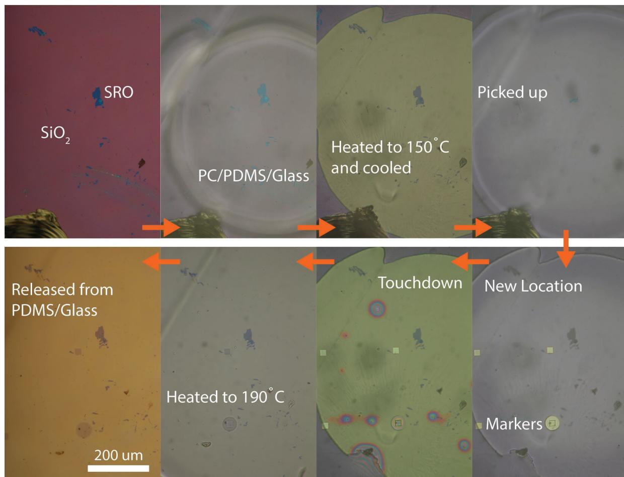
FIG. S9. Optical microscopy images of the flake pick-up process showing the transfer of non-annealed SRO from a dummy SiO<sub>2</sub>/Si substrate to a patterned substrate. Polycarbonate is used as a sticky polymer to transfer the flakes (in this case, SRO).
