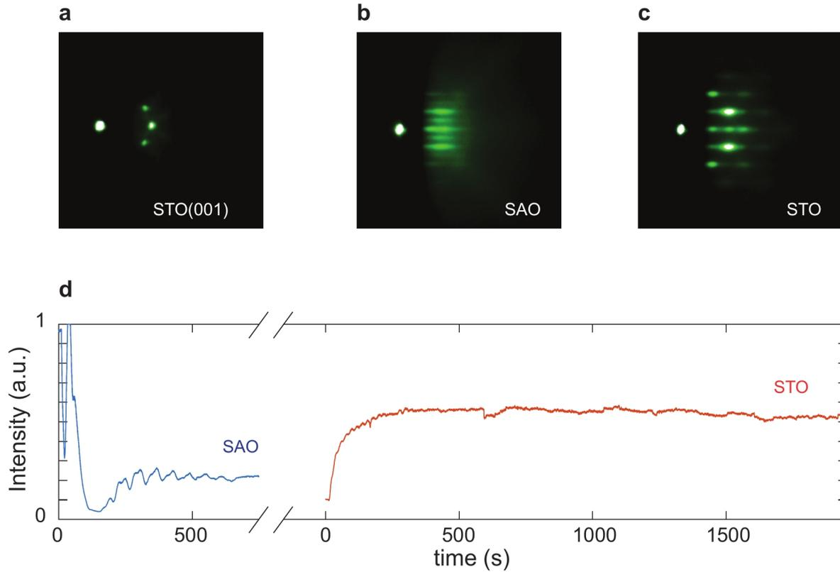
FIG. S1. Reflection high energy electron diffraction images of **a** the STO(001) substrate, **b** SAO buffer layer on STO(001), and **c** STO on SAO/STO(001). **d** RHEED oscillations of SAO and STO monitored during growth
