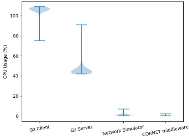
Fig. 6: CPU Usage of individual processes in Simulation
