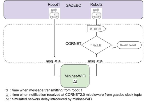
$t_1$  : time when message transmitting from robot 1
