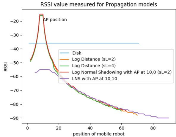
Fig. 8: RSSI measured from a single access point
