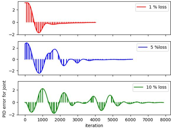
Fig. 10: Networked PID Controller error vs. Packet loss
