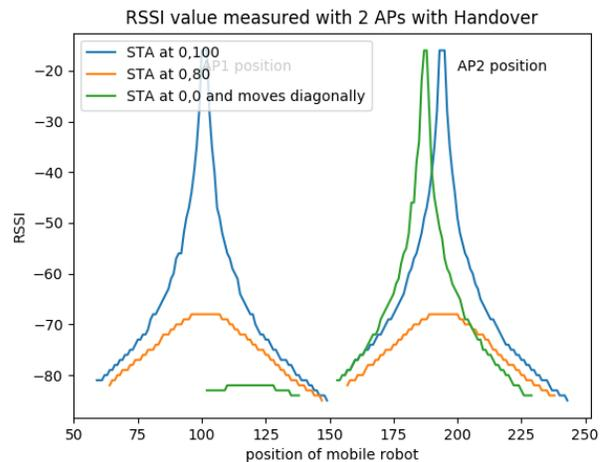
Fig. 9: RSSI measured with two access points (handover case)
