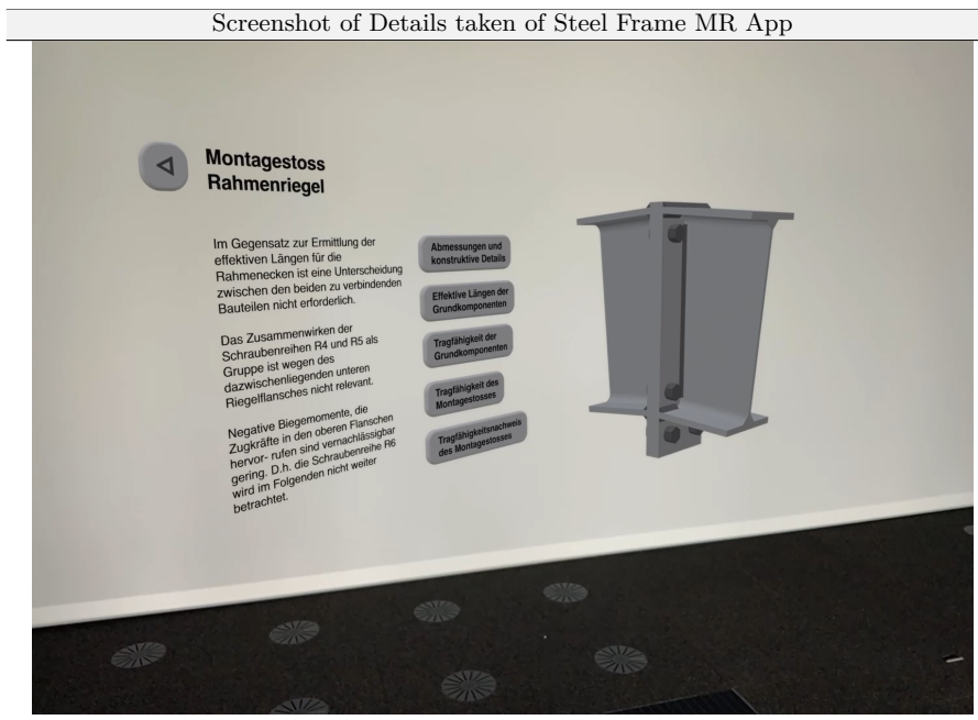
Fig. 11: Screenshot of Application B showing the explanatory instructions for designing the apex joints of the steel frame
