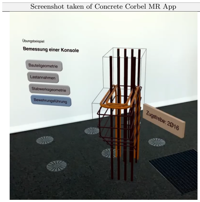
Fig. 9: Screenshot of Application A showing the rebar of the concrete corbel
