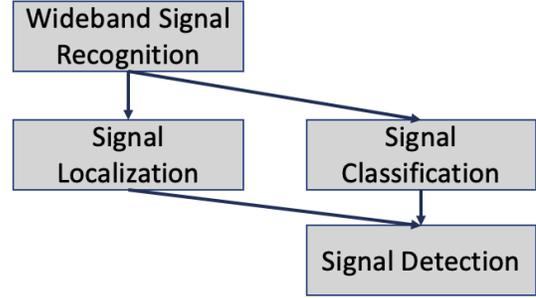
Fig. 1. Wideband Signal Recognition consists of signal classification and signal localization within time and frequency. Signal localization and signal classification depend on signal detection.
