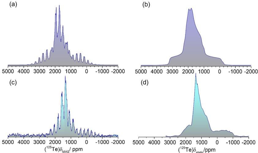
FIG. 7. DFT calculated and experimental solid-state NMR spectra of microcrystalline  $\text{WTe}_2$  at 9.4T. (a,b) The DFT calculated ssNMR spectra under magic angle spinning (a) and static (b) conditions. (c,d) The experimental ssNMR spectra under magic angle spinning (c) and static (d) conditions.
