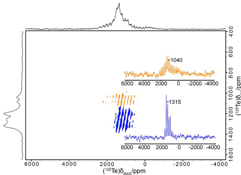
FIG. 9. The experimental  $^{125}\text{Te}$  MAS NMR aMAT spectrum at 14.1 T and 30 kHz MAS. The isotropic shifts and shift anisotropies of both Te(1),Te(3) and Te(2),Te(4) remain unchanged compared to the aMAT spectrum at 9.4 T.
