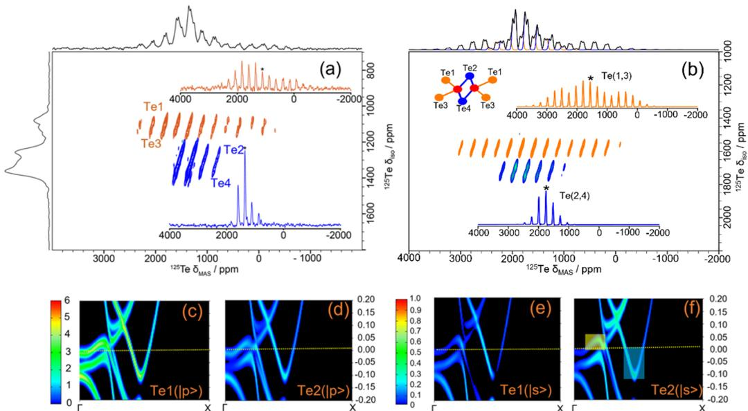
FIG. 2. (a) Experimental 2-D  $^{125}\text{Te}$  aMAT NMR spectrum at 30 kHz MAS in magnetic field of 9.4T. An equivalent spectrum at 14.1T is presented in Supplementary Figure 9. (b) DFT calculated 2-D  $^{125}\text{Te}$  aMAT NMR spectrum in the presence of SOC. (c-f) The relevant Te(1) and Te(2)  $|s\rangle$  and  $|p\rangle$  orbitals contribution to the k-resolved pDOS. Hole and electron pockets are highlighted in yellow, respectively blue color, in panel (f).
