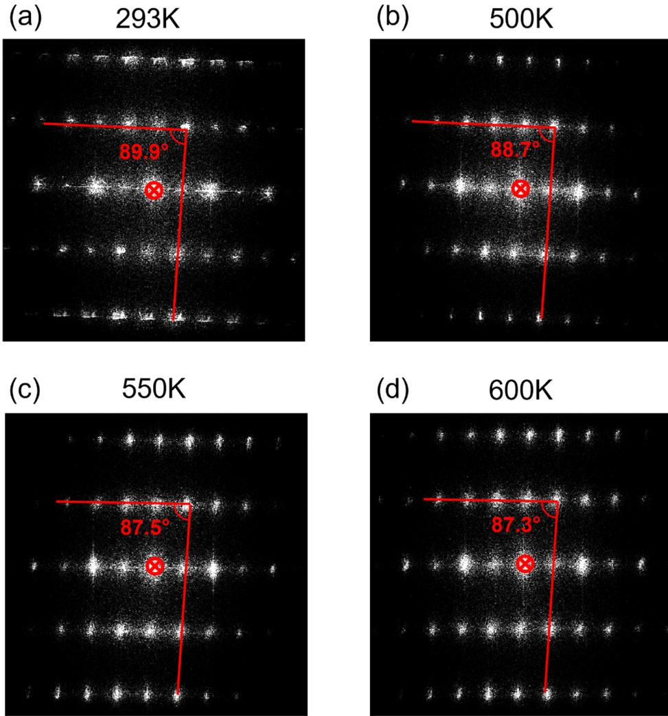
FIG. 5. Experimental electron diffraction patterns along the  $\langle 010 \rangle$  zone axis highlighting the structural phase transition from  $\gamma$ -WTe<sub>2</sub> to  $\beta$ -WTe<sub>2</sub>. (a-d) Experimental EDPs of WTe<sub>2</sub> at temperatures of (a) 293 K, (b) 500 K, (c) 550 K, and (d) 600 K.
