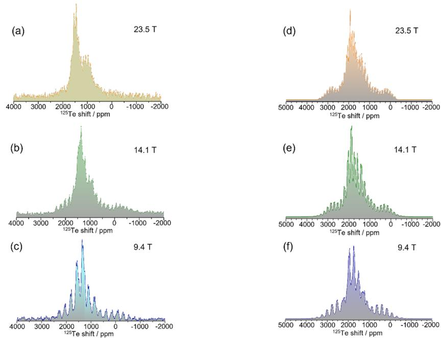
FIG. 8. Evolution of the  $^{125}\text{Te}$  MAS NMR spectral lineshape for varying magnetic field strength. (a-c) The experimental NMR lineshape for magnetic fields of 23.5 T, 14.1 T, and 9.4 T respectively. (d-f) The calculated NMR lineshape simulated for the same magnetic fields.
