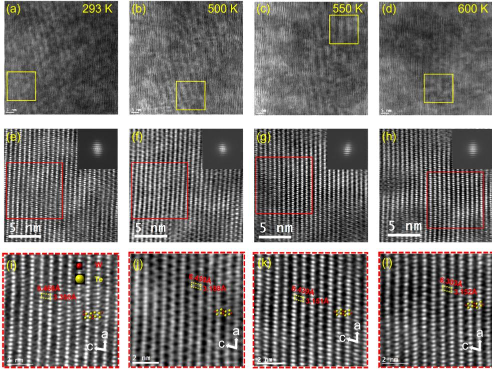
FIG. 3. HRTEM analysis of a plate-shaped particle in the microcrystalline  $\text{WTe}_2$  sample from room temperature (293K) up to 600K. (a-d) HRTEM of microcrystalline  $\text{WTe}_2$  along the  $[010]$  direction, at 293K, 500K, 550K, 600K. (e-h) Filtered Image and FFT data along the  $[010]$  direction for the same temperatures. The red rectangle highlights the areas expansions of which are presented in (i-l) to showcase the change in the crystal lattice parameters upon heating.
