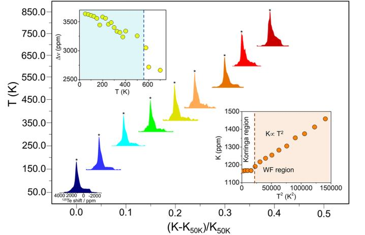
FIG. 4.  $^{125}\text{Te}$  static NMR spectra in the temperature range 50K – 700K. Calibration in the frequency axis is performed according to the  $K$ -values of the most intense resonance as indicated by the star. The upper left inset shows the half height full width  $\Delta\nu$  of the broad signal component assigned to the Te(1), Te(3) atomic sites. The lower right inset presents  $K$  vs.  $T^2$ .
