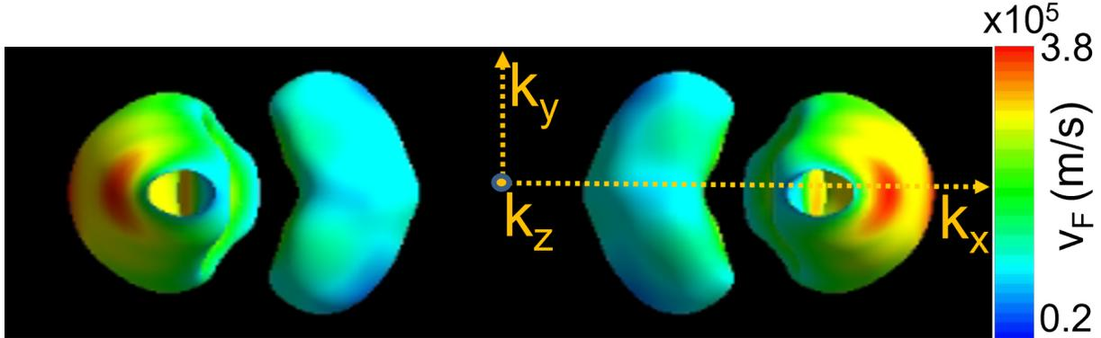
FIG. 12. The Fermi velocity map across the hole and the electron pockets in the  $T_d$  phase of  $WTe_2$ .
