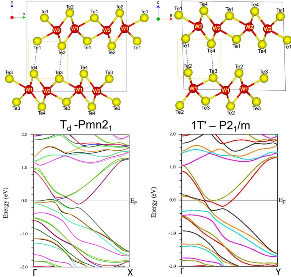
FIG. 6. The unit cells and the electron energy band structures of the  $\text{WTe}_2$   $T_d$ - $\text{Pmn}2_1$  and  $1T'$ - $\text{P}2_1/m$  crystal phases, along the lines connecting the high symmetry points  $\Gamma \rightarrow X$  and  $\Gamma \rightarrow Y$ , respectively.
