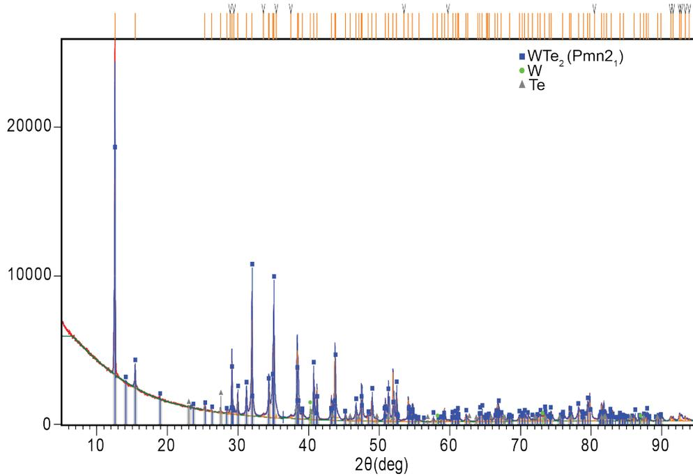
FIG. 1. The experimental X-ray powder diffraction patterns (red) and the Rietveld analysis (blue) of microcrystalline  $\text{WTe}_2$  crystallized in the orthorhombic  $\text{Pmn}2_1$  space group (S.G. #31). Traces of elemental W (green) and Te (gray) are also observed.
