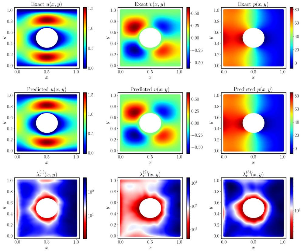
Figure 25: *Stokes equation*: Predicted solution of the best trained physics-informed DeepONet for one example in the test data-set.
