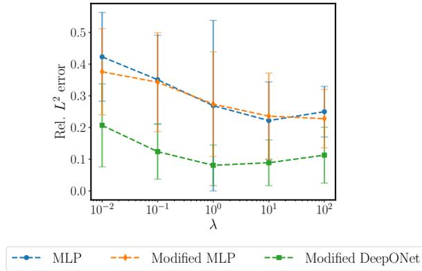
Figure 20: *Burger's equation*: Relative  $L^2$  error of physics-informed DeepONets represented by different architectures and trained using different fixed weights  $\lambda_{bc} = \lambda_{ic} = \lambda \in [10^{-2}, 10^2]$ , averaged over the test data-set.
