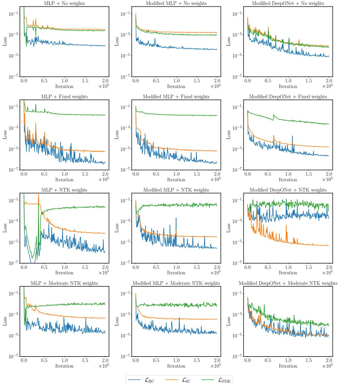
Figure 19: *Burger's equation*: Training loss convergence of a DeepONet models using different DeepONet architectures and weighting schemes for  $2 \times 10^5$  iterations of gradient descent using the Adam optimizer. Here we remark that all losses are unweighted.
