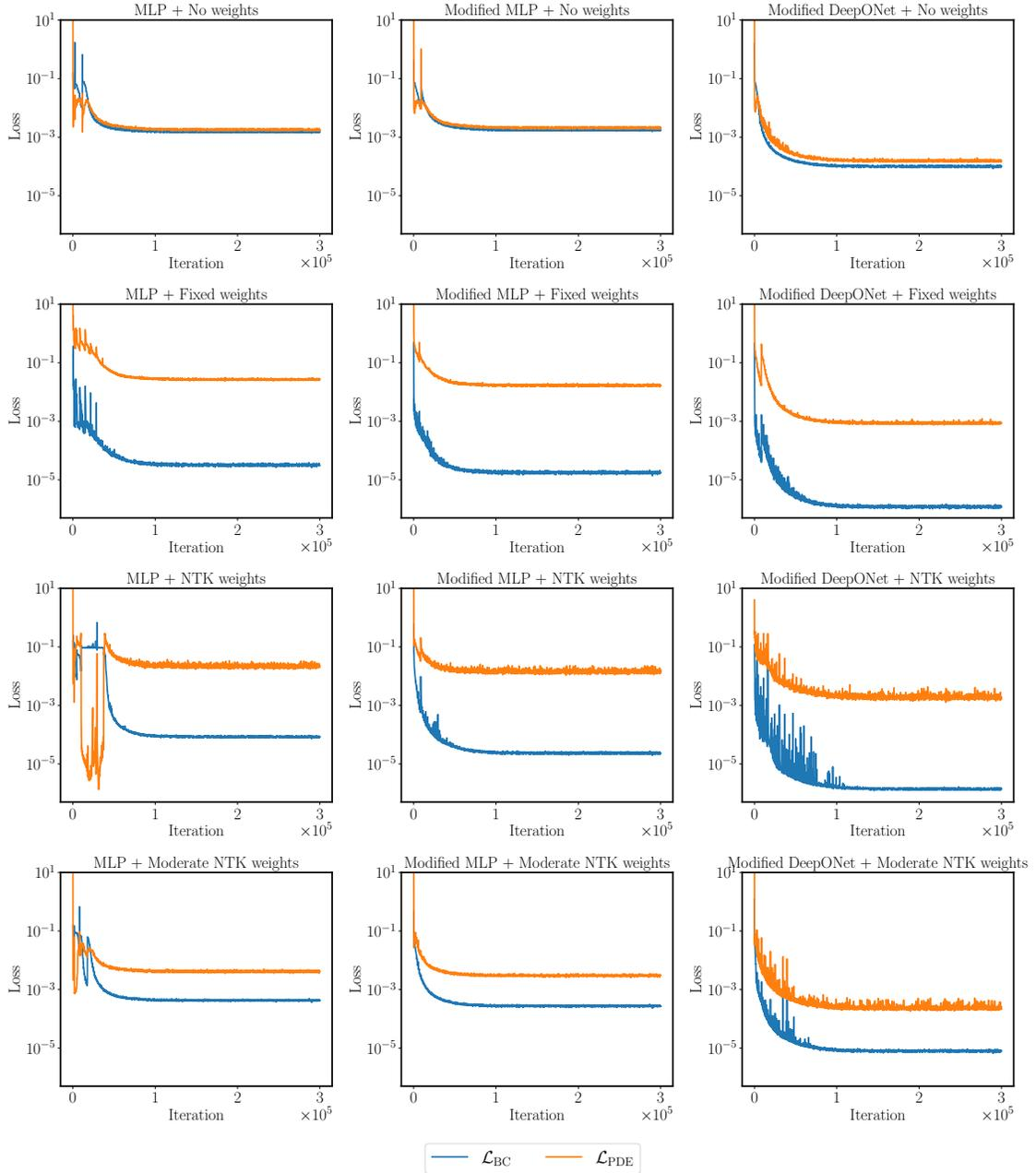
Figure 16: *Advection equation*: Training loss convergence of a DeepONet models using different DeepONet architectures and weighting schemes for  $3 \times 10^5$  iterations of gradient descent using the Adam optimizer. Here we remark that all losses are unweighted.
