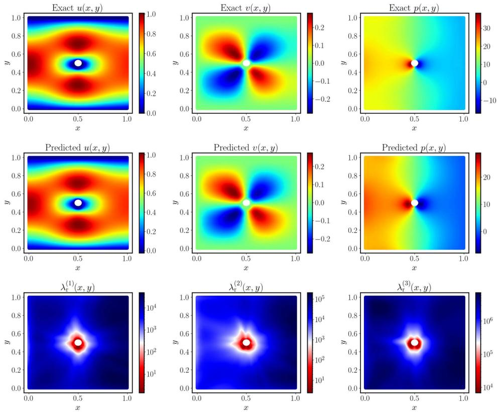
Figure 27: Stokes equation: Predicted solution of the best trained physics-informed DeepONet for one example in the test data-set.
