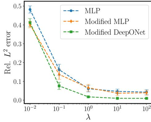
Figure 17: *Advection equation*: Relative  $L^2$  error of physics-informed DeepONets represented by different architectures and trained using different fixed weights  $\lambda_{bc} = \lambda_{ic} = \lambda \in [10^{-2}, 10^2]$ , averaged over the test data-set.
