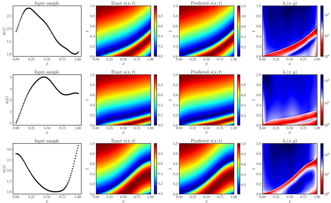
Figure 18: *Advection equation*: Predicted solution of the best trained physics-informed DeepONet for three different examples in the test data-set.
