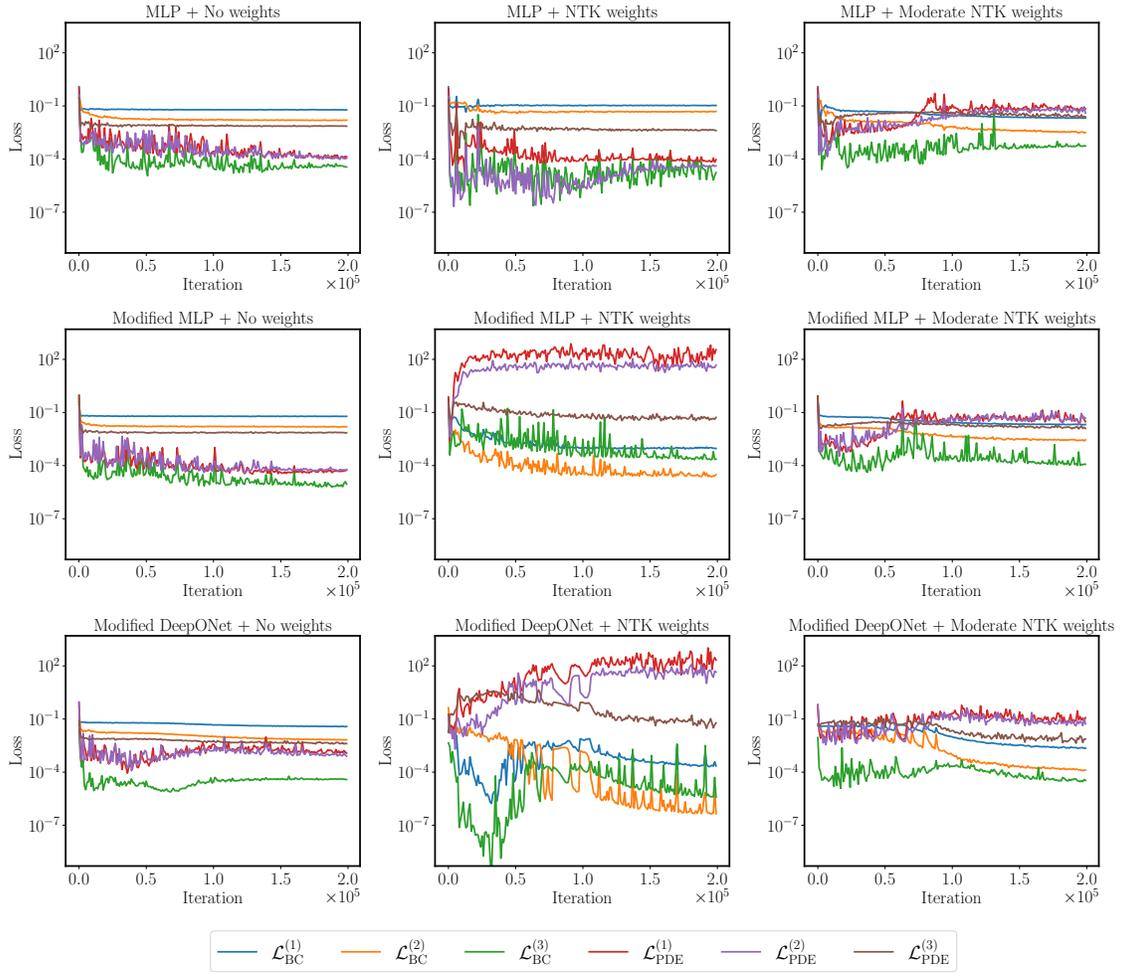
Figure 24: *Stokes equation*: Training loss convergence of a DeepONet models using different DeepONet architectures and weighting schemes for  $2 \times 10^5$  iterations of gradient descent using the Adam optimizer. Here we remark that all losses are unweighted.
