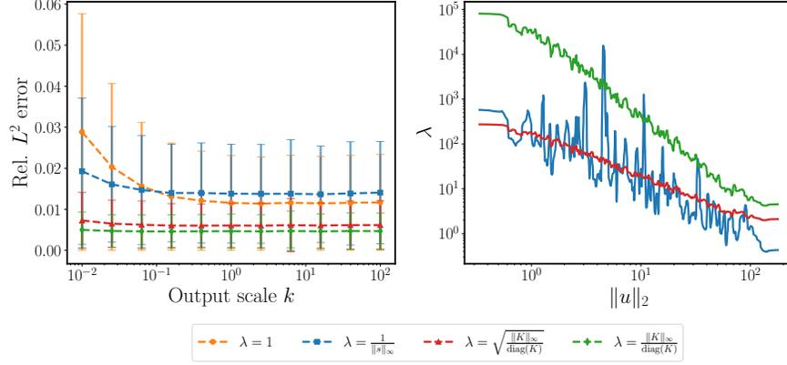
Figure 4: *Anti-derivative operator*: *Left*: Mean and standard deviation of the relative  $L^2$  prediction errors of the trained DeepONets using different weighting schemes, averaged over the test data sampled from a GRF with different output scale  $k \in [10^{-2}, 10^2]$ . A detailed description of the legend is summarized in Table 2. *Right*: Weight distributions of trained models with different weighting schemes in increasing order of  $\|u\|_2$ .
