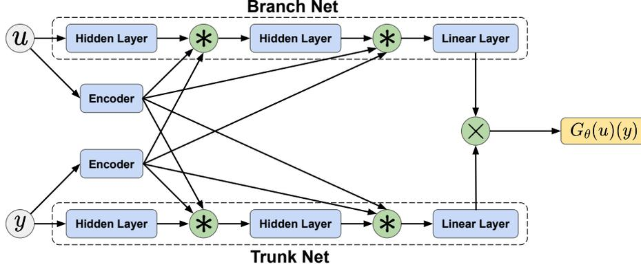
Figure 5: *Modified DeepONet architecture*: Two encoders are applied to the input samples and the input coordinates, respectively. The embedded features are then inserted into each hidden layer of the branch network and the trunk network using a  $*$  operation, which is defined in equation (3.26) - (3.27). The final outputs is obtained by the same way as conventional DeepONets, i.e, merging the outputs of the branch and trunk networks via a dot production.
