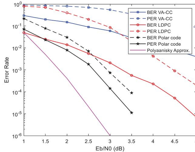
**Figure 10:** Error rate vs.  $E_b/N_0$  for  $K = 128$  bits
