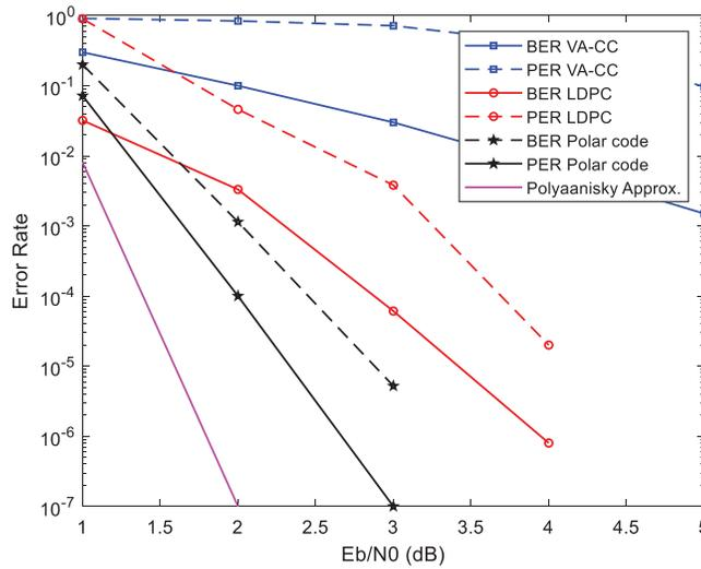
**Figure 8:** Error rate vs.  $E_b/N_0$  for  $K = 512$  bits
