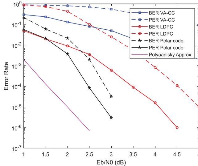
**Figure 9:** Error rate vs.  $E_b/N_0$  for  $K = 256$  bits
