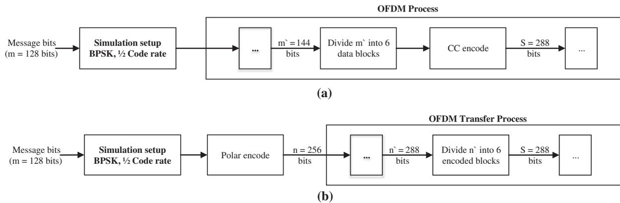
**Figure 5:** PHY layer simplified diagram of encoding 128 message bits by using CCs versus polar codes considering BPSK modulation and code rate at 1/2. (a) CC encoding process (b) Polar encoding process
