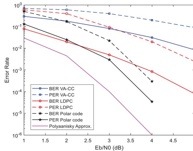
**Figure 11:** Error rate vs.  $E_b/N_0$  for  $K = 64$  bits
