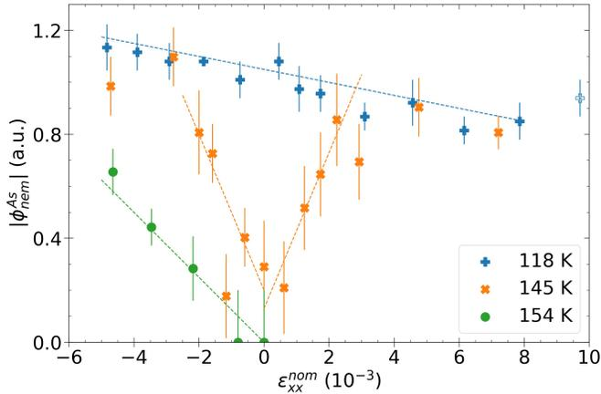
FIG. 4: Strain dependence of the As phonon derived nematic order parameter  $|\phi_{nem}^{As}|$  at three temperatures around  $T_S$ . The dashed lines are guides to the eye and not fits of the data. The empty symbol at 118 K at high tensile strain indicates that we suspect that the sample broke at this point.
