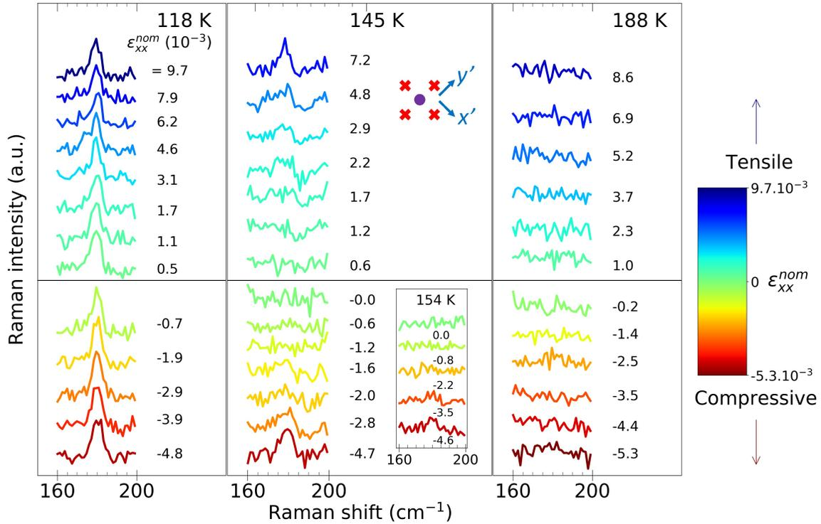
FIG. 3: Strain dependence of the As phonon Raman spectra in the  $x'y'$  polarization configuration at four temperatures around  $T_S$ . Note that crystal likely broke during the last measurement at 118 K under strong tension  $\epsilon_{xx}^{nom} = 9.7 \times 10^{-3}$ . This precluded measurements at 154 K under tension: only spectra under compression are shown.
