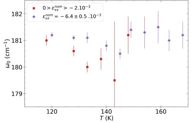
FIG. 8: Temperature dependence of the effective phonon energy  $\omega_0$  as extracted from the Fano lineshape fitting. At low strain the fitting above 148 K yielded very high error bars for  $\omega_0$  due to the very weak phonon intensity and the corresponding values are not shown.
