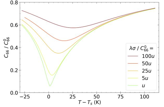
FIG. 10: Temperature dependence of the shear modulus  $C_{66}$  under increasing  $B_{2g}$  stress  $\sigma$ . Here we have used  $T_S = 138$  K,  $T_0 = 100$  K,  $u = 1$ ,  $a = 1$  and  $C_{66}^0 = 30$  GPa
