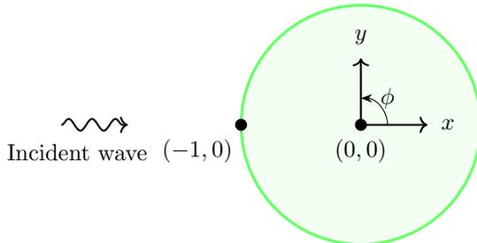
Figure 3: Schematic for the circular cylinder scattering problem
