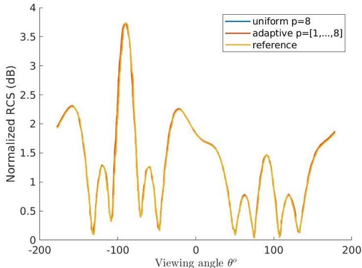
Figure 21: RCS, 2 adjacent cylinders,  $\phi = 90^\circ$
