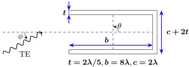
Figure 11: Schematic for the semi-open cavity problem
