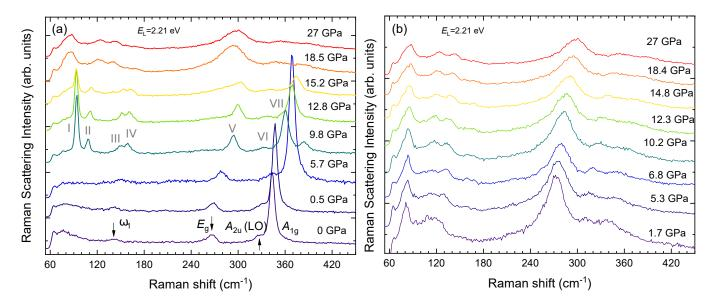
FIG. 2. Raman scattering spectra of bulk  $HfS_2$  as a function of hydrostatic pressure for compression (a) and decompression (b) cycle
