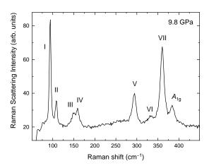
FIG. 4. Raman scattering spectrum of bulk  $HfS_2$  in hydrostatic pressure of 9.8 GPa.
