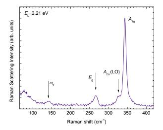
FIG. 1. Raman scattering spectrum of bulk HfS<sub>2</sub> at ambient pressure.
