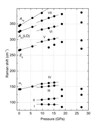
FIG. 3. The evolution of the Raman scattering peak energies in bulk  $HfS_2$  with hydrostatic pressure. Straight lines correspond to linear fits to experimental data.
