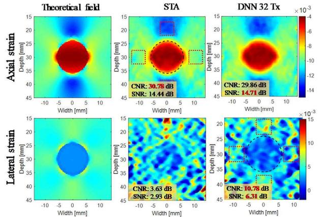
Fig. 4. Axial and lateral strains obtained from different imaging methods, as well as the corresponding theoretical fields. The applied strain is -1%. White Gaussian noise with an SNR of -10 dB is added to STA data and noise with the same power is added to apodized PW data. The black circle and red blocks are ROI and background regions used for CNR calculation, respectively.
