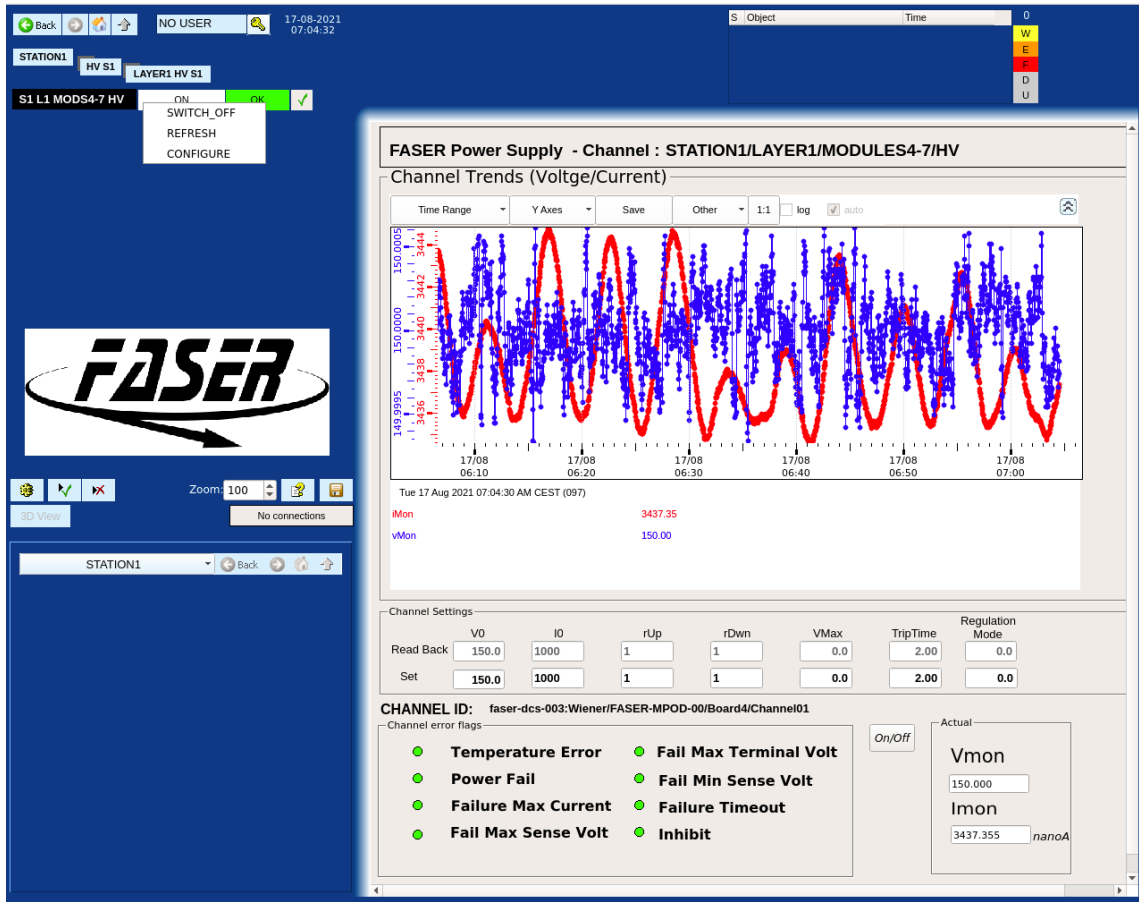
Figure 17. A DCS FSM panel via which the low and high voltage of a tracker station is controlled.
