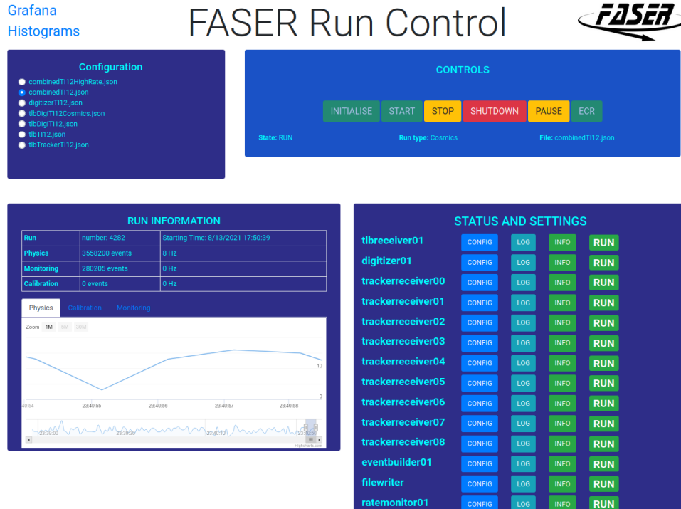
Figure 12. Example screen shot of the RCGui web application during cosmic ray data taking with the FASER detector.
