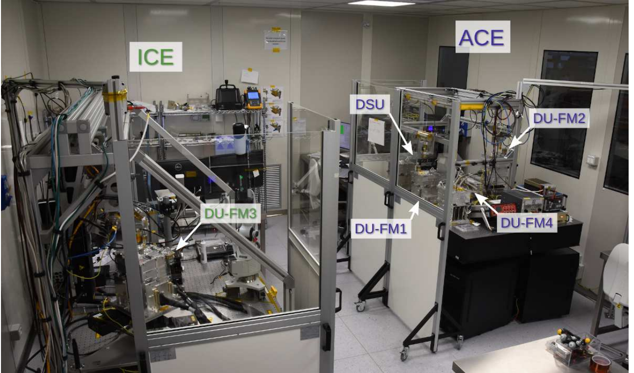
Figure 2: Overview of the two calibration stations, named ICE and ACE, in the ISO 7 (class 10,000) IXPE clean room at INAF-IAPS during the contemporaneous calibration of the third DU flight model (DU-FM3) on the ICE and the Instrument testing with DSU-EM and DU-FM1, DU-FM2 and DU-FM4 on the ACE. Shields are used to limit the X-ray exposure of operators.
