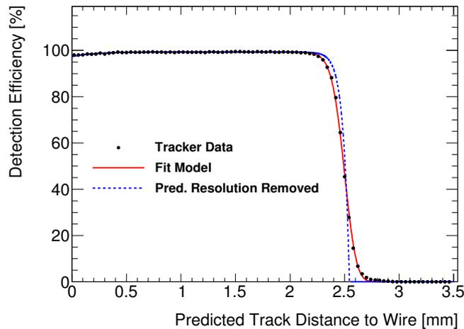
**Figure 23:** Straw detection efficiency measured as a function of distance of the interpolated track prediction from the wire. The red solid line is a fit model of exponential decreases from a constant efficiency at the wire and straw edges, and includes the intrinsic resolution from the track position prediction. The blue dotted line is the same function after deconvolution of this resolution.
