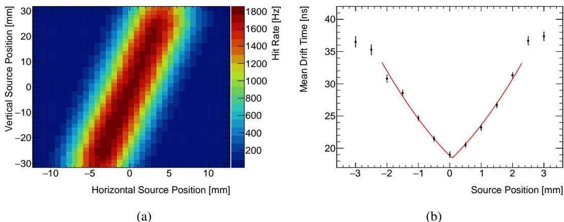
**Figure 19:** (a) Two-dimensional distribution of event rate versus horizontal and vertical position for a single straw. All straws except the straw of interest have been disabled. (b) Average drift time versus  $^{90}\text{Sr}$  source position for a single straw. The slope of the fit (red line) is the time to drift distance relationship and the minimum of the fit is the wire position.
