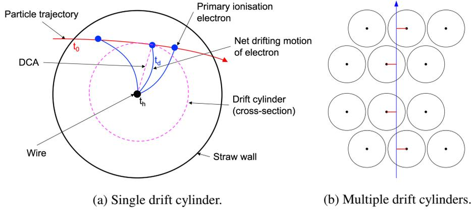
**Figure 1:** Top-down depiction of the drifting of primary ionization electrons to the straw wire, the DCA reconstructed from the drift time  $t_d$  and the subsequent drift cylinder specified by the DCA. Also shown are the measured hit time  $t_h$  and the time that the charged particle traversed the straw  $t_0$ .
