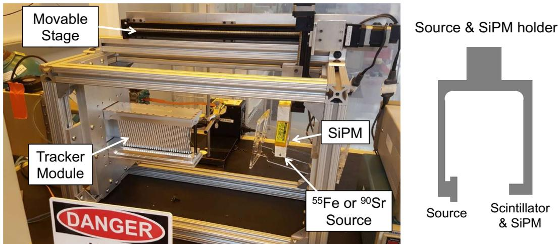
**Figure 16:** A photograph of a tracking detector module installed in the test stand and a diagram showing the source and detector holder. The movable stages are at the top of the frame. The radioactive source and a scintillator trigger are mounted on an inverted “U”-shaped aluminum bracket attached to the vertical movable stage. A detailed description of the test stand design is given in [15].
