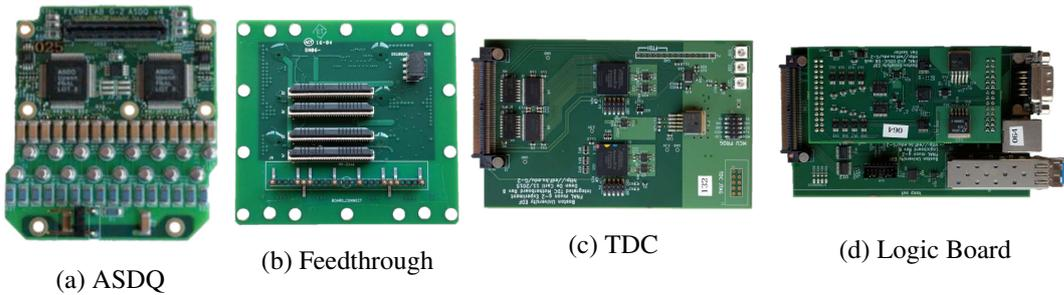
**Figure 14:** Four of the different types of frontend electronics boards. The functionality of each board is described in the text.
