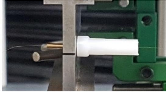
(b) Machine crimping the 'long' pins.
