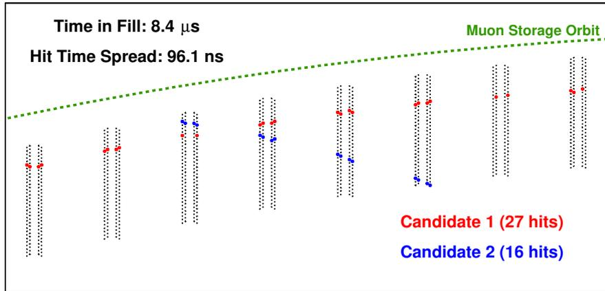
**Figure 24:** An event display of a time island with multiple track candidates in the tracking detector. Each wire is marked with a black dot and the hits are marked with larger circles. The color of each hit designates the candidate to which it has been assigned. The longer, straighter track (red circles) is likely a muon lost from the storage region, and the shorter, more curved track (blue circles) is a decay positron.
