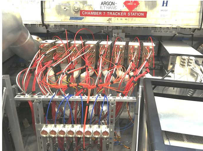
**Figure 20:** One of the two tracking detector stations installed in the muon storage ring vacuum chamber. Eight modules can be seen, connected to red HV cables, orange optical fibers and silver power cables. Red gas tubes enter at the top of each module, air cooling is attached with white tube below. At the front of the photo, the flow meters for the water-cooling system are visible.
