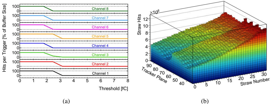
**Figure 21:** (a) The number of hits per trigger as a function of the ASDQ discriminator threshold. At low thresholds, where noise dominates, the hit rate is large enough to fill the storage buffers. Above 3.5 fC the noise rate is negligible. (b) The number of hits per channel for all straws over a three-day data-taking period. No channels have significantly more than any other, demonstrating sufficiently low noise levels.
