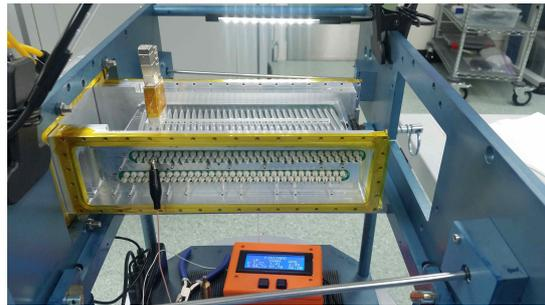
(f) A tension test being carried out on a wire.
