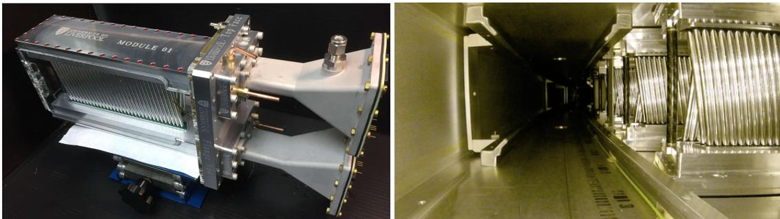
(b) The first completed tracking detector module. (c) Tracking detector modules installed in the storage ring vacuum chamber.
