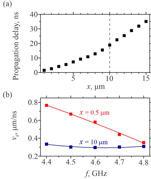
FIG. 4. Spatial dependence of the propagation delay measured for a 20-ns long spin-wave pulse at the carrier frequency  $f=4.5$  GHz. Vertical dashed line marks the end of the transition region. Frequency dependence of the group velocity at the beginning of the transition region ( $x=0.5 \mu\text{m}$ ) and at its end ( $x=10 \mu\text{m}$ ), as labelled. Symbols – experimental data. Curves – guide for the eye. The data are obtained at  $H_0=1000$  Oe.
