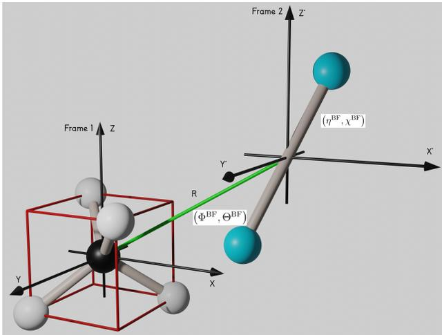
**Figure 2.** Body-fixed coordinate frame of the  $\text{CH}_4\text{-N}_2$  complex.
