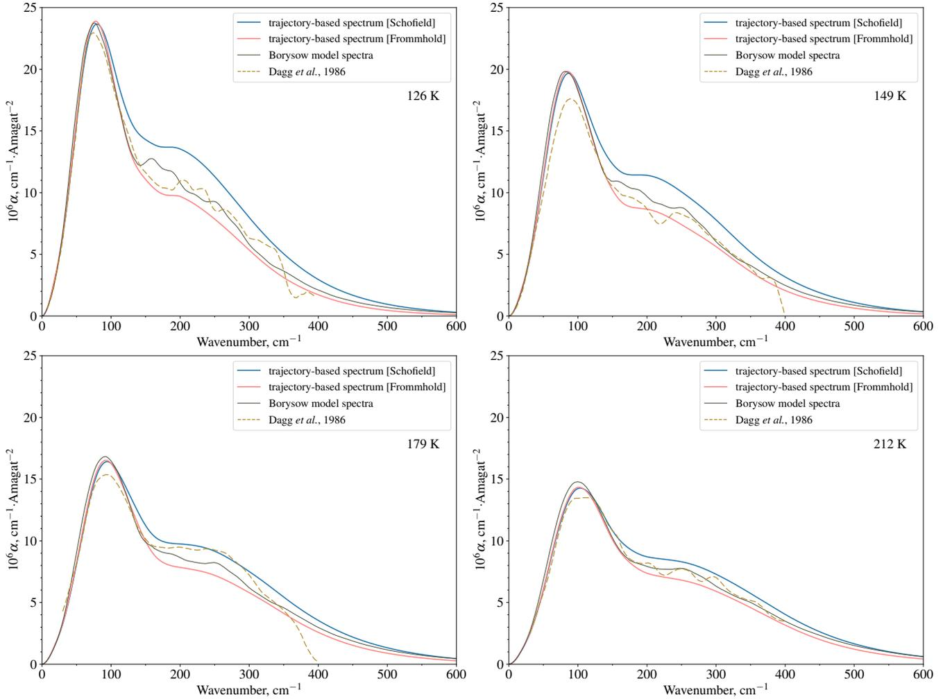
**Figure 6.**  $\text{CH}_4\text{-N}_2$  collision-induced absorption spectra at selected temperatures. Dashed yellow lines denote experimental measurements by Dagg et al. (1986) at 126, 149, 179, and 212 K. The blue and red lines indicate the trajectory-based results obtained using Schofield’s and Frommhold’s quantum correction factors. Model profiles of Borysov & Tang (1993) are represented with gray lines.
