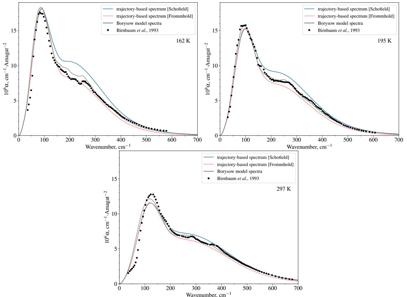
**Figure 7.** CH<sub>4</sub>-N<sub>2</sub> collision-induced absorption spectra at selected temperatures. Markers denote experimental data by Birnbaum et al. (1993) at 162, 195, and 297 K. The blue and red lines indicate the trajectory-based results obtained using Schofield’s and Frommhold’s quantum correction factors. Model profiles of Borysov & Tang (1993) are represented with gray lines.
