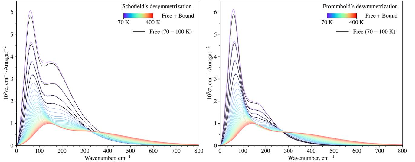
**Figure 4.**  $\text{CH}_4\text{-N}_2$  CIA spectral profiles corresponding to both bound and unbound states (in color) from 70 to 400 K with a step of 10 K. The black lines represent profiles corresponding to unbound states at 70–100 K. The left panel shows profiles subjected to Schofield’s quantum correction factor, whereas Frommhold’s correction is utilized for the profiles on the right panel.
