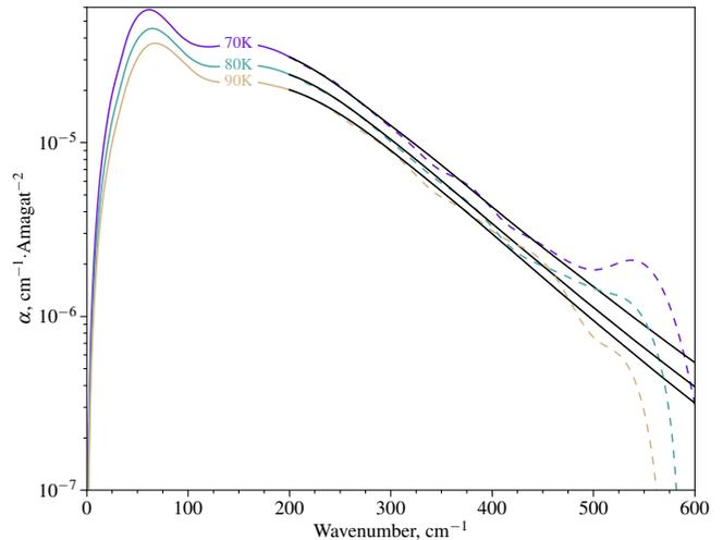
**Figure 3.**  $\text{CH}_4\text{--N}_2$  CIA spectral profiles corresponding to unbound states obtained through TCFs processing (in color) and through formalism (14) (in black) at 70–90 K. Both sets of profiles utilize Schofield’s quantum correction factor. The TCF-based profiles longward of  $200$   $\text{cm}^{-1}$  are shown with dashed lines. Resultant profiles are obtained upon the stitching of two sets at  $200$   $\text{cm}^{-1}$ .
