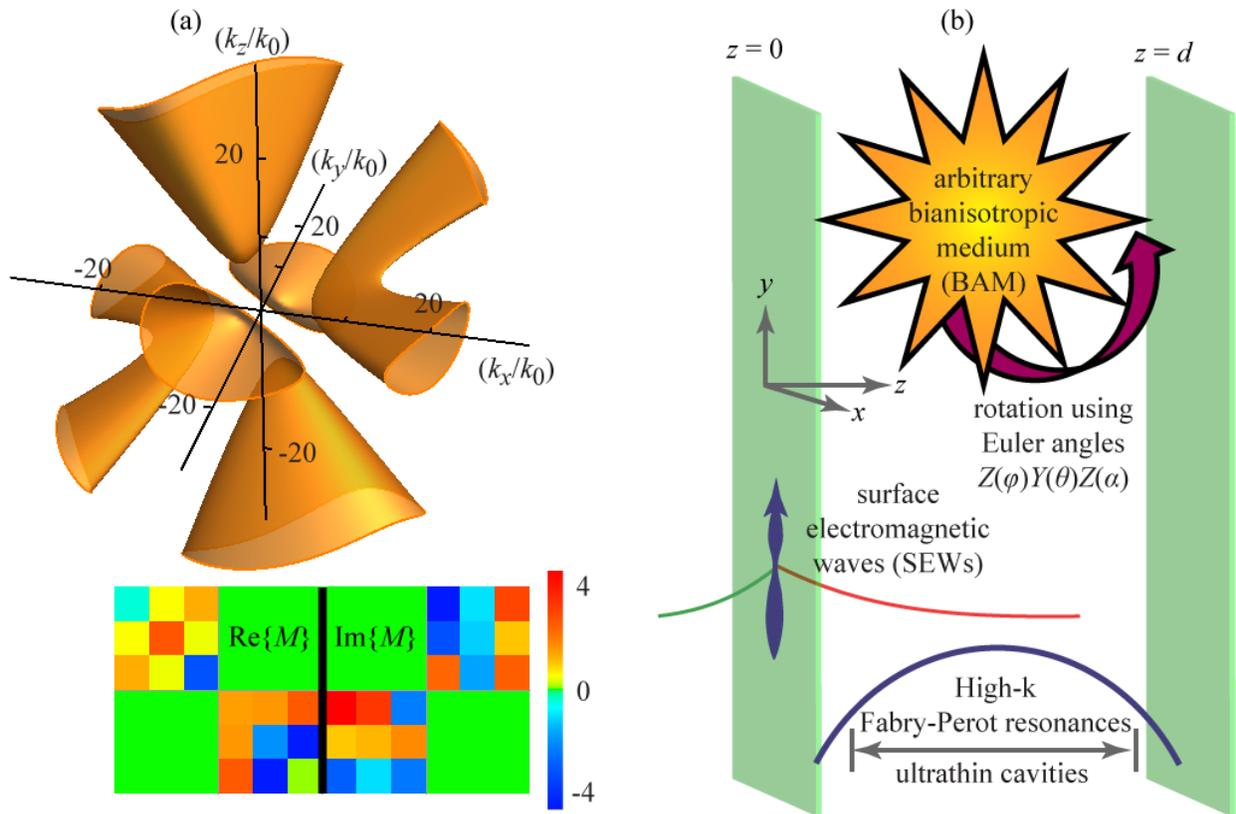
Fig. 1. (a) Isofrequency Fresnel wave surface in  $k$ -space for a tetrahyperbolic bianisotropic material with  $\hat{M}$  matrix illustrated with color coding in the bottom of the panel. (b) Schematic illustrating the conventions in this paper as described in the text.
