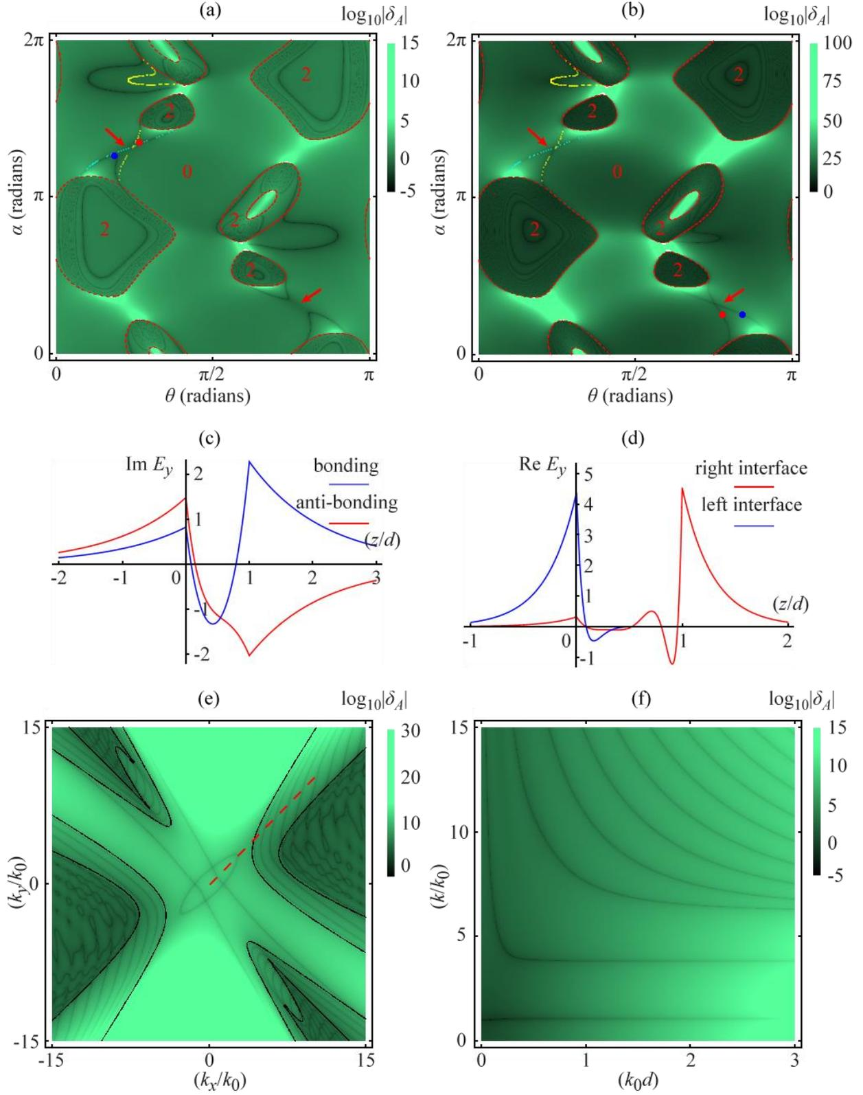
Fig. 3. Surface Electromagnetic Waves in Bianisotropic Media. (a-b) The resonant denominator  $\delta_A$  as a function of the bianisotropic material orientation with respect to the layer boundaries for  $q_x = 2$  and
