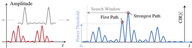
Figure 3: The CIR is calculated based on the received signal and a local template of the expected signal. A correlation peak indicates high similarity. However, with multi-path effects, there are multiple peaks. The receiver identifies the first LoS path, e.g., by searching back in time from the strongest peak.
