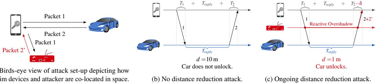
Figure 6: Overview of a distance reduction attack (a). Two devices determine their relative distance with UWB HRP by measuring the ToF of packets 1 and 2 (b). The attacker cannot decrease distance by sending 1 or 2 in advance because their content is unpredictable (STS). Instead, the attacker reactively overshadows 2 with 2' (c). Packet 2' is crafted to inject noise that the victim receiver interprets as an earlier copy of 2, decreasing distance.
