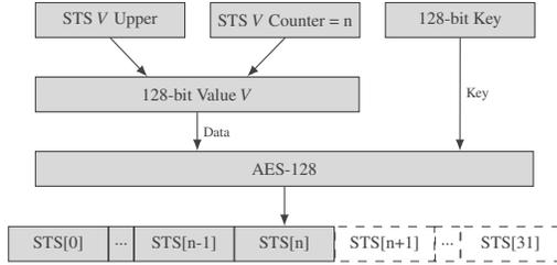
Figure 5: Cryptographically secure STS generation with AES in counter mode. Each iteration results in a random 128-bit block. The STS  $V$  Counter is incremented for every iteration. The entire STS comprises 32 blocks, or 4096 bits [4].
