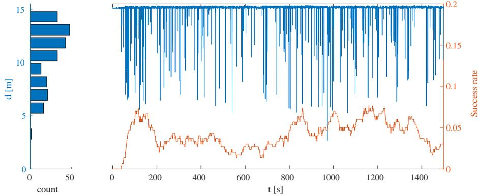
Figure 10: A 25 min trace of raw distance measurements (iPhone–iPhone, 15 m) under attack with two devices. The left part is a histogram of those measurements that report reduced distances. The overall rate of successful distance reductions is 4.08 %.
