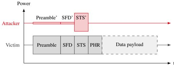
Figure 7: The attacker overshadows the legitimate signal (gray) with a carefully crafted attack packet (red). The attacker's STS' is random, without knowing the victim's STS.
