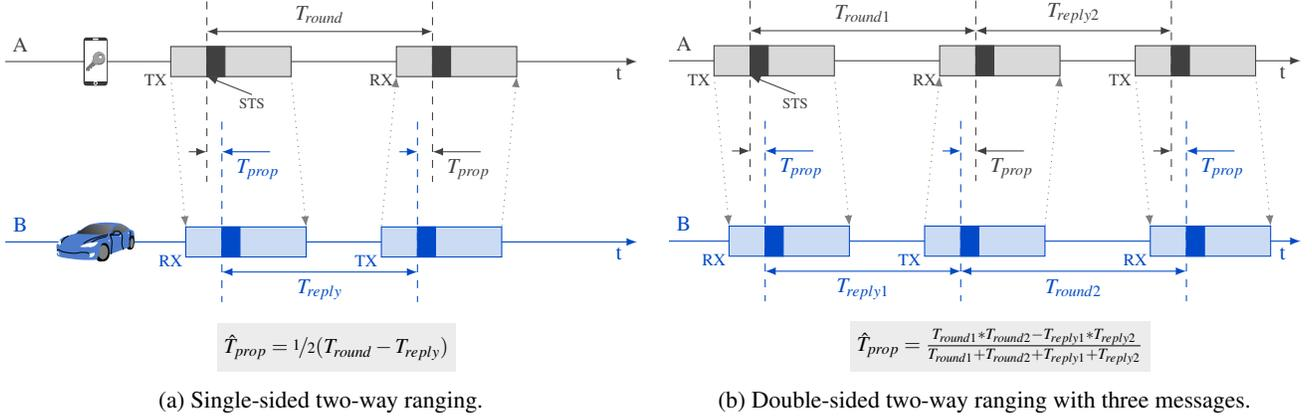
Figure 1: The principle of two-way ranging [4].
