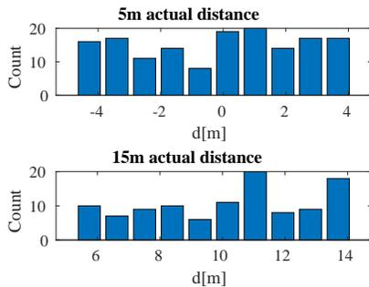
Figure 11: Distribution of reduced distance reports for the iPhone–iPhone (5 m and 15 m) setup, attacked with single device over a 15 min observation period. The overall rate of successful distance reductions is ca. 2.2 % in both cases.
