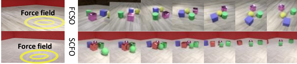
Figure 5: Left: DRoom simulation environment setup where yellow rings denote the force fields. Right: One fast-camera-slow-object (FCSO) sample ( top row ) and slow-camera-fast-object (SCFO) sample ( bottom row ). Both are randomly selected from the DR-Lvl.3 dataset.
