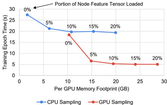
Figure 11. Multi-GPU MAG240M training time comparison while loading different amounts (in %) of node feature tensor into GPU memory. GPU sampling requires the graph structure to be loaded in GPU memory and thus it has a higher memory footprint.
