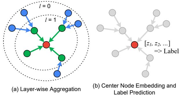
Figure 1. GNN with node feature aggregation and label prediction.
