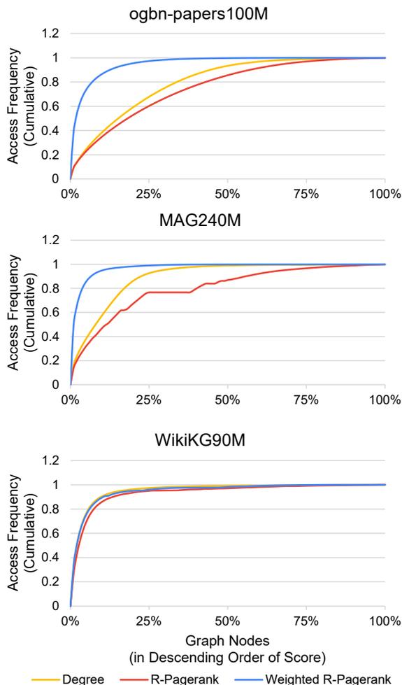
Figure 7. Access frequency distribution comparison on different datasets with different score functions. Y-axis is normalized to the total number of access.
