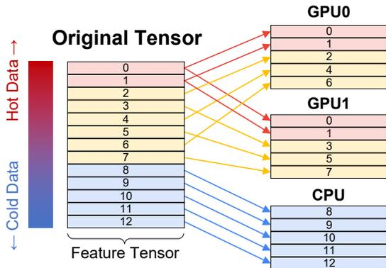
Figure 6. Data loading in multi-GPU environment.
