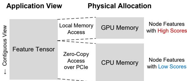
Figure 4. Simple data placement and access method overview.
