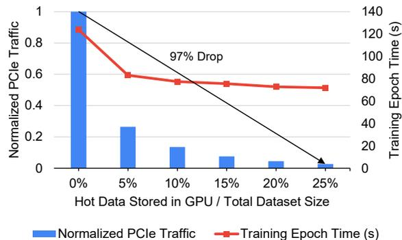
Figure 10. PCIe traffic and training time comparison in actual GNN training with increasing hot data portion loaded in GPU. ogbn-papers100M dataset used.
