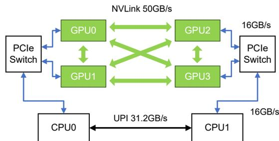
Figure 5. An example system with four NVIDIA V100 GPUs connected over NVLink. All bandwidth numbers shown are unidirectional.
