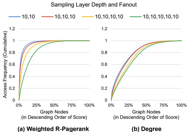
Figure 9. Access frequency distribution comparison of using different neighbor sampling parameters in ogbn-papers100M dataset.
