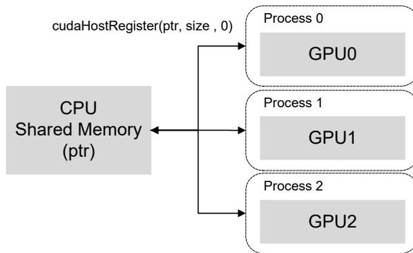
Figure 12. `cudaHostRegister()` is used to map memory space allocated in CPU into GPU. `cudaHostRegister()` needs to be called by all processes individually.
