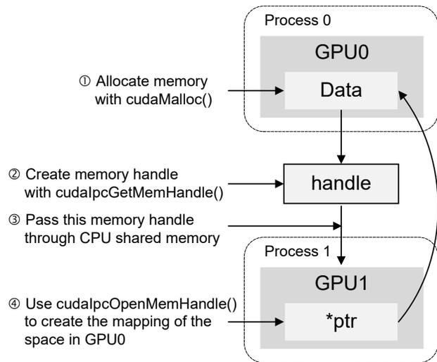
Figure 13. Peer-to-Peer GPU memory sharing mechanism in multiprocessing setup.
