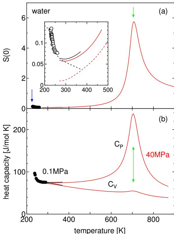
FIG. 9. (a)  $S(0)$  parameter and (b) specific heat capacities of liquid and supercooled liquid water. The red and black lines denote  $S(0)$ ,  $C_P$ , and  $C_V$  at 40 MPa and 0.1 MPa, respectively, calculated using the IAPWS-95 formula [43]. The black circles denote experimentally obtained values of  $S(0)$  [18] under the vacuum condition and  $C_P$  [50] at 0.1 MPa. The dashed lines are visual guides.
