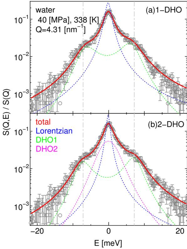
FIG. 11. Fitting results of the dynamic structure factor of liquid water at 40 MPa, 338 K, and  $Q = 4.31 \text{ nm}^{-1}$ , by (a) 1-DHO and (b) 2-DHO model. The gray circles and solid red line represent the experimental and fitting results, respectively. The dashed blue, green, and pink lines represent the Lorentzian, DHO1, and DHO2 components, respectively. The vertical gray dot-dashed line represents the energy of DHO1 in 2-DHO model.
