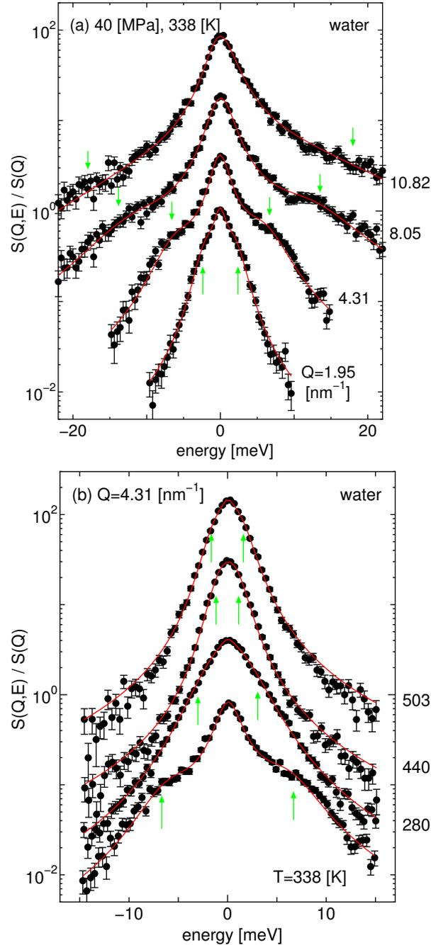
FIG. 10. Normalized dynamic structure factor of liquid water. (a)  $Q$  variation at 40 MPa and 338 K, and (b)  $T$  variation at  $Q=4.31 \text{ nm}^{-1}$ . The  $Q$  and  $T$  values are indicated in the figure. Each spectrum is slightly shifted for clarity. The green arrows represent the excitation energies determined by 1-DHO analysis.
