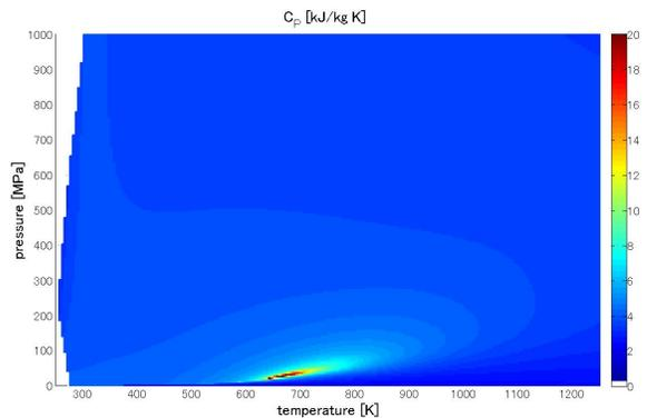
FIG. 8. Contour map of isobaric heat capacity  $C_P$ .
