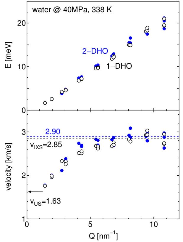
FIG. 12. (a) Dispersion curve of excitation energy and (b)  $Q$ -dependent sound velocity for liquid water. The black open and blue closed circles correspond to 1-DHO and 2-DHO models, respectively.  $v_{\text{IXS}}$  is determined in the selected  $Q$ -range ( $7.5 < Q < 11 \text{ nm}^{-1}$ ).  $v_{\text{US}}$  is the sound velocity calculated using the IAPWS-95 formula [43].
