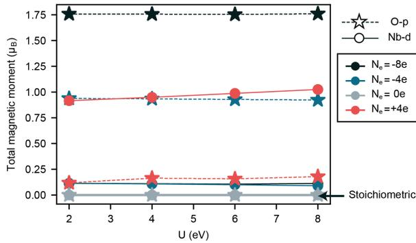
FIG. S1. The dependence of the species-dependent total magnetic moment as a function of the effective Hubbard U parameter for both stoichiometric and off-stoichiometric configurations of B-Nb<sub>2</sub>O<sub>5</sub>. Electron and hole doping is included by adding a compensating background charge to the *ab initio* calculation.
