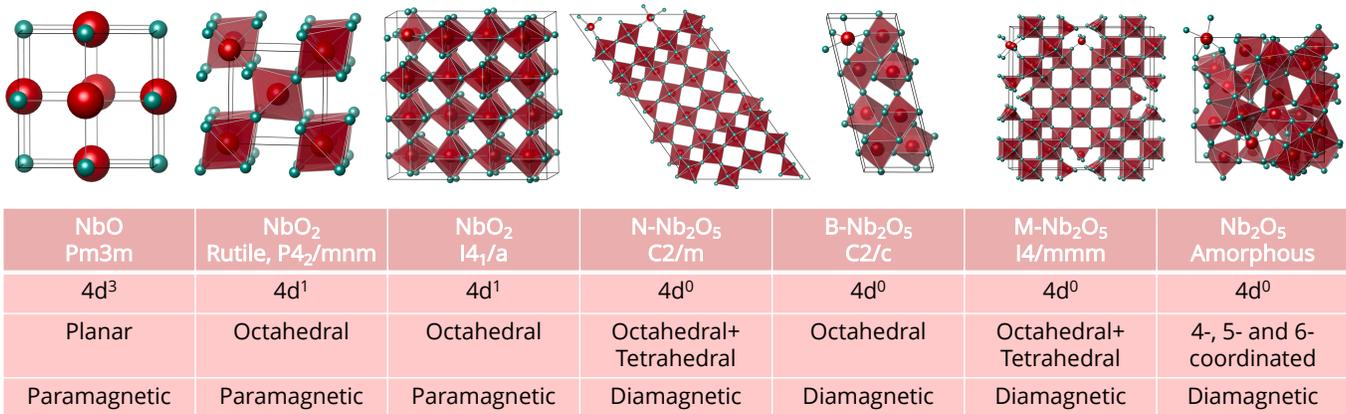
FIG. 1. Crystal structures of the Nb oxides considered in this work with their nominal valence configuration on the Nb atoms, the Nb coordination environment(s) and the resulting magnetic order in the stoichiometric case.
