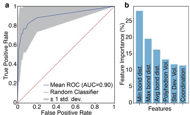
FIG. S8. (a) Receiver-operating characteristic curve of a random forest model trained to classify if an ion is magnetic depending on local environment descriptors of the amorphous configurations. (b) Histogram of feature importance (percentage) of a pruned set of descriptors.
