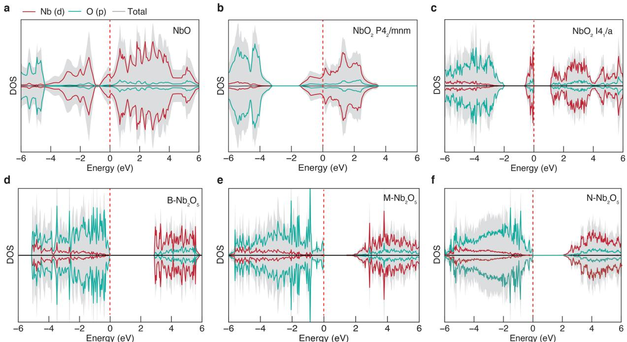
FIG. S3. The total and orbital-projected density of states for the (a) NbO ( $Pm\bar{3}m$ ), (b) NbO<sub>2</sub> ( $P4_2/mmm$ ), (c) NbO<sub>2</sub> ( $I4_1/a$ ), (d) B-Nb<sub>2</sub>O<sub>5</sub>, (e) M-Nb<sub>2</sub>O<sub>5</sub> and (f) N-Nb<sub>2</sub>O<sub>5</sub>. The Fermi level is indicated by the dashed red line. Nb ( $d$ ) states are illustrated by the solid red line, O ( $p$ ) by the solid teal line and the Total Density of states by the grey shaded area.
