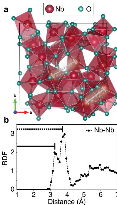
FIG. S7. (a) Example of an amorphous configuration (configuration no. 5) obtained after quenching a molecular dynamics snapshot. Solid and dashed lines represent Nb-Nb distances between edge-sharing and point-sharing polyhedra, respectively. (b) Radial distribution function obtained from all quenched molecular dynamics snapshots. The peaks are labelled solid and dashed lines from panel a.
