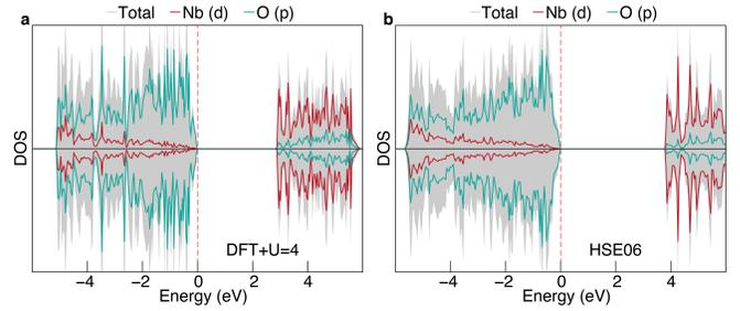
FIG. S2. Comparison between PBE+U=4 eV and HSE06 for B-Nb<sub>2</sub>O<sub>5</sub>. The experimental bandgap is estimated to be 3.8 – 3.9 eV<sup>7</sup>
