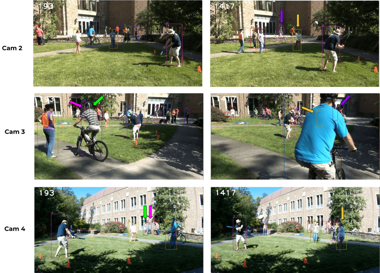
Figure 9. Qualitative tracking results in the Garden 1 in Campus dataset at three overlapping camera views (zoom in for better visualization). The benefit of the multi-camera approach can be found in two typical situations. First, at frame 193 (left column), two objects at the pink and green arrows in Cam 3 were not visible in this view; however, we could overcome these missing positions by using information from Cam 4. Similarly, at frame 1417, two objects at yellow and purple arrows are occluded in Cam 3. Fortunately, leveraging visible detections in Cam 4 and Cam 2, we can continue tracking these objects.
