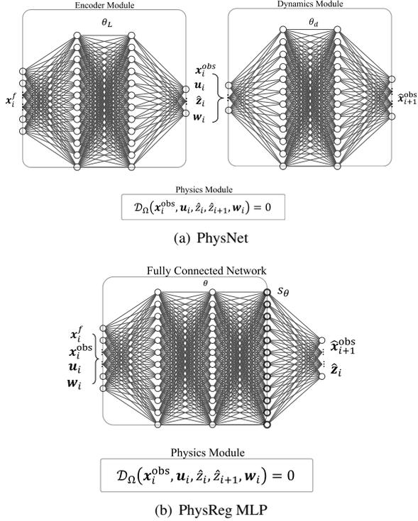
Figure 1: Physics Informed Neural Network architectures.  $\mathbf{x}_i^f$  represents a high dimensional feature engineered state component of the system, whereas  $\mathbf{x}_i^{\text{obs}}$  represents the observable components of the input sample  $i$ .  $\mathbf{z}_i$  represents a low-dimensional latent representation of the system.
