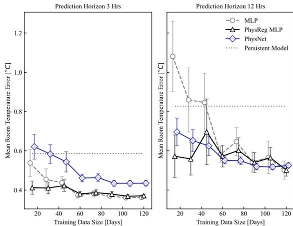
Figure 6: Mean room temperature prediction error for varying training data size. The plots represent mean error of 20 trained models and the error bars represent  $\pm$  standard deviation. The models used in this experiment are trained and tested on real-world data obtained from a cold storage unit.
