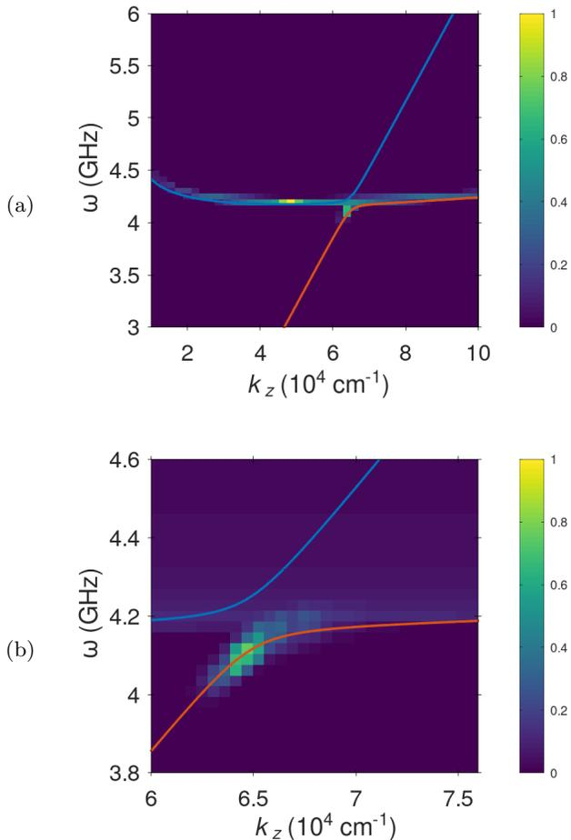
FIG. 5. Magnon density  $\rho_{km}$  as function of the wave vector  $\mathbf{k} = e_z k_z$  parallel to the external field and the excitation frequency  $\omega$ , normalized to the value of the magnon condensate. The dispersion relations of the upper (+) and lower (-) magnetoelastic modes for wave vectors parallel to the external magnetic field are indicated as blue and red lines respectively. The left peak in (a) is due to the magnon condensate. (b) shows a close-up of the hybridization area.
