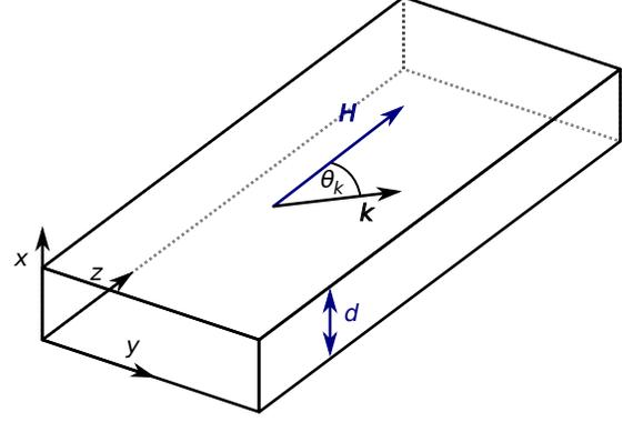
FIG. 1. Geometry of a thin YIG film with thickness  $d$  in the presence of a uniform external magnetic field  $\mathbf{H} = H\mathbf{e}_z$  parallel to the plane of the film. In this work we consider only the lowest, uniform thickness modes with in-plane wave vectors  $\mathbf{k} = \mathbf{e}_z |\mathbf{k}| \cos \theta_{\mathbf{k}} + \mathbf{e}_y |\mathbf{k}| \sin \theta_{\mathbf{k}}$ .
