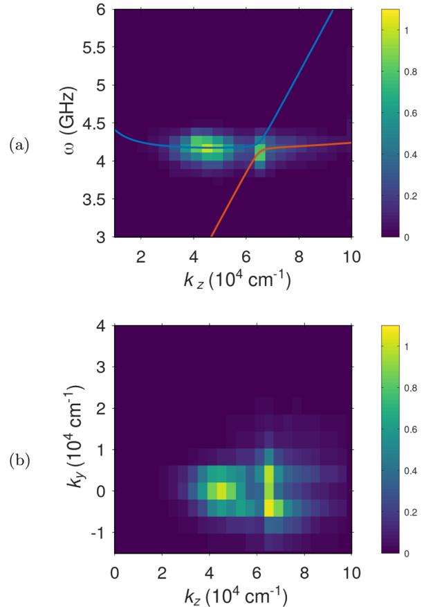
FIG. 8. (a) Experimental magnon-phonon spectra and the population of the lowest magnon mode, with the dispersion relations of the upper (+) and lower (-) magnetoelastic modes for wave vectors parallel to the external magnetic field indicated as blue and red lines, respectively. (b) Wave vector-resolved magnon population. Both plots are normalized to the value of the magnon condensate to facilitate direct comparison with the theoretical prediction in Fig. 5.
