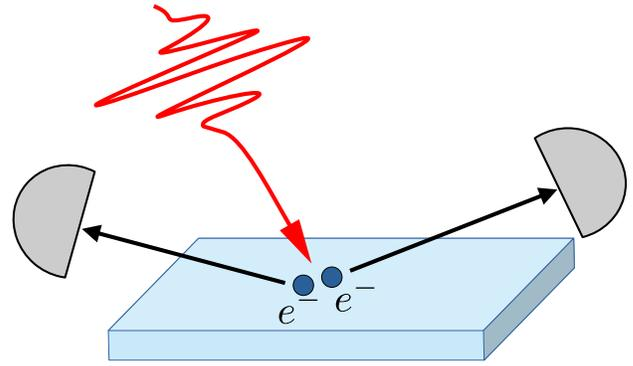
FIG. 1. Schematic of the ARPFS setup: An electromagnetic pulse is hitting onto the  $\mathcal{PT}$ -symmetric superconductor. Electrons are emitted from the substrate due to interaction with photons from the pulse and are registered by two detectors located at opposite sides of the sample. The aim of the detection scheme is to identify correlated electrons that formed a Cooper pair in the sample before they have left it.
