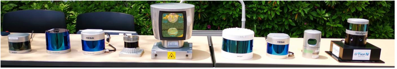
Figure 5: Multiple 3D LiDARs, from Velodyne, Hesai, RoboSense, Ouster, etc.
