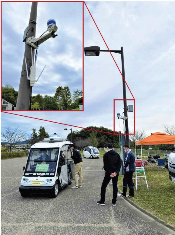
Figure 20: V2I infrastructures at Morikoro park in Nagoya, Japan. A self-driving vehicle interacting with the road side units (RSU). Inset: A LiDAR deployment on a pole. Images courtesy of Mr. Abraham Monrroy-Cano of Perception Engine Inc.
