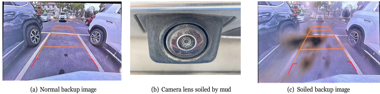
Figure 17: Contamination effect on a Cadillac XT5 back-up camera. The mud contamination is formed naturally from off-road driving after rain. Vehicle testing and images courtesy of Mr. Dawei Wang, Pan Asia Technical Automotive Center Co., Ltd.
