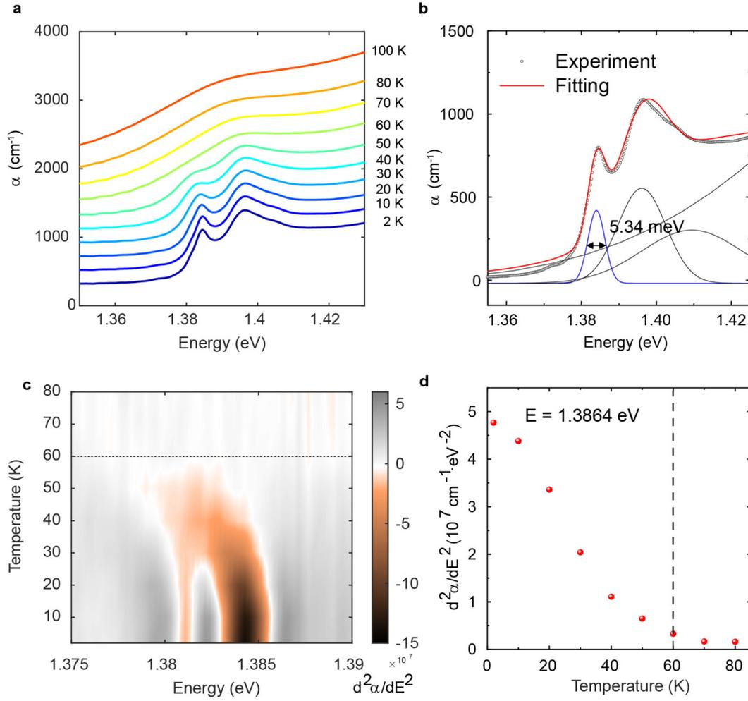
**Figure 2.** Absorption spectra of NiI<sub>2</sub> single crystal. a) The in-plane absorption coefficient of single-crystal NiI<sub>2</sub> in the ferroelectric spiral (proper screw) phase at various temperatures. b) Model fitting curves of the absorption coefficient at T = 2 K. c) Second derivative of the absorption coefficient with respect to energy. d) Value of the second derivative at E = 1.3864 eV as a function of temperature. The dotted lines in c) and d) indicate  $T_{N2} = 59.5$  K.
