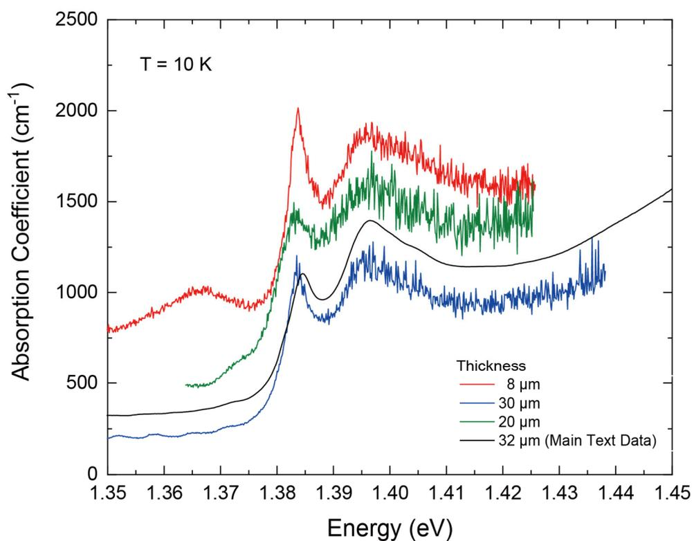
**Figure S2.** Thickness-dependent absorption spectra measured at  $T = 10$  K. All absorption experiments show the exciton at  $1.384$  eV with the same linewidth. Absorption coefficient calculation is dependent on the thickness of the sample, so there may be an error in absorption coefficient due to an error in the sample thickness. However, the feature of the exciton (like a position, a linewidth) is consistently seen regardless of the thickness of the sample.
