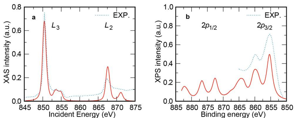
**Figure S4.** Theoretical and experimental data of XAS and XPS. a) Theoretical x-ray absorption spectroscopy (XAS) and b) core-level x-ray photoemission spectroscopy (XPS) spectra of NiI<sub>2</sub> cluster calculated with parameters presented in Table 1. Dotted lines in a) and b) refer to the experimental spectra of XAS and XPS, respectively. Experimental XPS spectra were taken after previous literature<sup>[1]</sup>.
