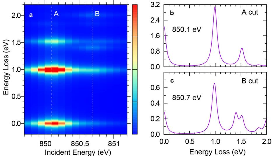
**Figure 5.** Theoretical data of RIXS. a) The theoretical Ni  $L_3$ -edge resonant inelastic x-ray scattering (RIXS) map. The Ni  $L_3$ -edge RIXS intensity as a function of the energy loss when the incident x-ray energy is b) 850.1 eV (A cut in a) and c) 850.7 eV (B cut).
