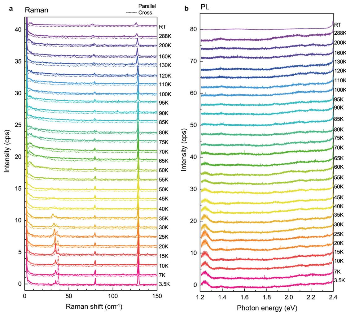
**Figure S3.** Raman and PL spectra of bulk  $\text{NiI}_2$ . a) Raman spectra depicted by solid (dashed) lines are the results of parallel (cross) polarization configuration. b) PL spectra don't have any signal around the position of the absorption peak  $\sim 1.38$  eV.
