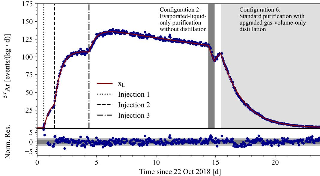
Fig. 5: Fit online distillation model to argon data: Three  $^{37}\text{Ar}$  injections into the GXe volume led to an increase in  $^{37}\text{Ar}$  events inside the LXe volume. The event evolution during *C1* (*Standard purification without distillation*) (white), a short period *C2* (*Evaporated-liquid-only purification without distillation*) (dark grey), and *C6* (*Standard purification with upgraded gas-volume-only distillation*) (light grey) is described by  $x_L$ .
