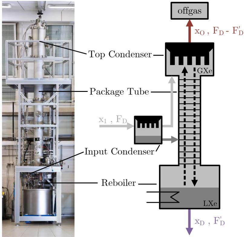
Fig. 2: (Left) Distillation column in the University of Münster before shipment to LNGS. (Right) Scheme of the distillation process showing the in-coming and out-going krypton concentrations  $x_i$  and xenon flows  $F_i$  as described in the text.
