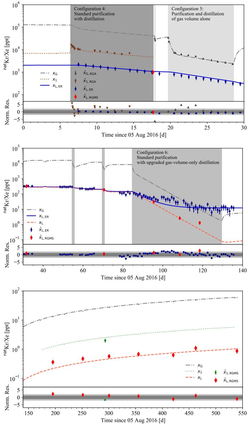
Fig. 4: Fit online distillation model to krypton data: The fit curves are labeled as  $x_i$ , while the different measurements are denoted by  $\hat{x}_i$ . The fit results are presented in three panels. Normalized residuals are shown in the bottom of each panel. Grey bands visualize the  $1\sigma$  and  $2\sigma$  deviation.
