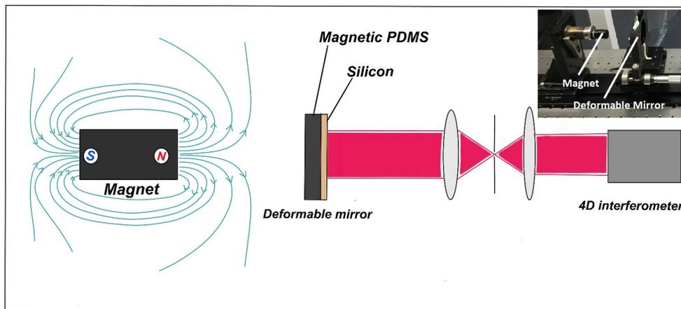
**Fig. 4** Illustration showing the experimental setup used for measuring the surface deformation at the silicon (Si) layer side of PMADM. The image at the top right corner is a snapshot of the laboratory setup showing the magnets and the PMADM on a moving stage. By changing the relative distance between the magnets and the PMADM sample, we can vary the magnetic load subjected on the PMADM structure.
