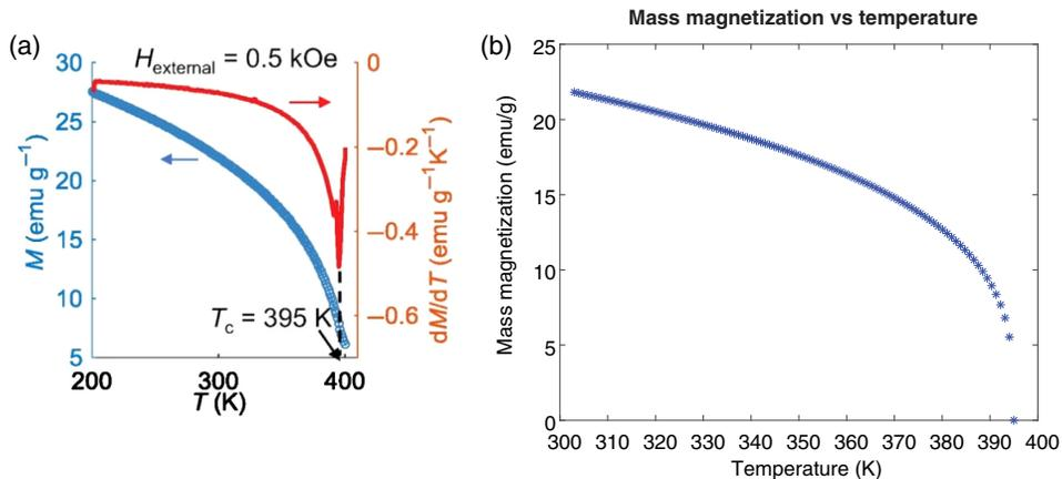
**Fig. 2** (a) Plot of mass magnetization versus temperature taken from Fig. 2D of Li et al.<sup>42</sup> (b) Plot of mass magnetization versus temperature governed by Eq. (1) taken from Fig. 2 of Jha et al.<sup>45</sup> The relationship describes the decreasing magnetization properties of the composite structure with increasing temperature. The magnetization comes to zero when the temperature is equal to the Curie temperature.
