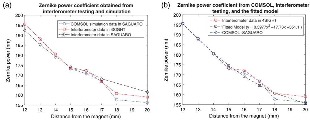
**Fig. 12** (a) Comparison between Zernike power term coefficients obtained from experimental laboratory testing (4SIGHT and SAGUARO) and our FEM model (COMSOL + SAGUARO) for our PMADM. (b) A curve fitted with 1.8382 nm RMSE (1.12%) predicts the nonlinear trend of the Zernike power term coefficient with varying separation distance between the magnets and the PMADM when the laser is off.
