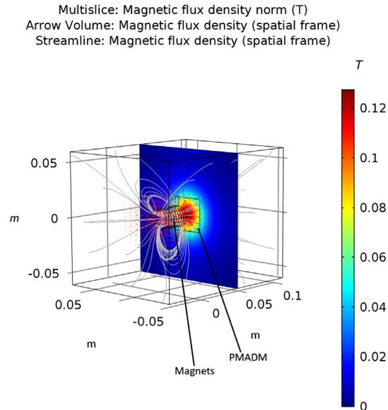
**Fig. 5** COMSOL simulation of eight magnets subjecting a magnetic load on the PMADM structure. The magnetic field lines (in gray) and the magnetic flux density at the C-layer of the PMADM are shown. The separation between the magnet and the PMADM is 12 mm, and a maximum flux density of 0.12 T can be seen at the C-layer of the PMADM.
