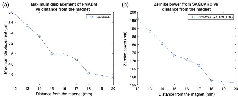
**Fig. 7** (a) Plot showing simulation of maximum displacement with changing separation distance between the magnet and the PMADM. (b) Zernike power term plot obtained from postprocessing the displacement maps obtained from COMSOL in SAGUARO. An optical pupil diameter of 8 mm is considered in the calculation.
