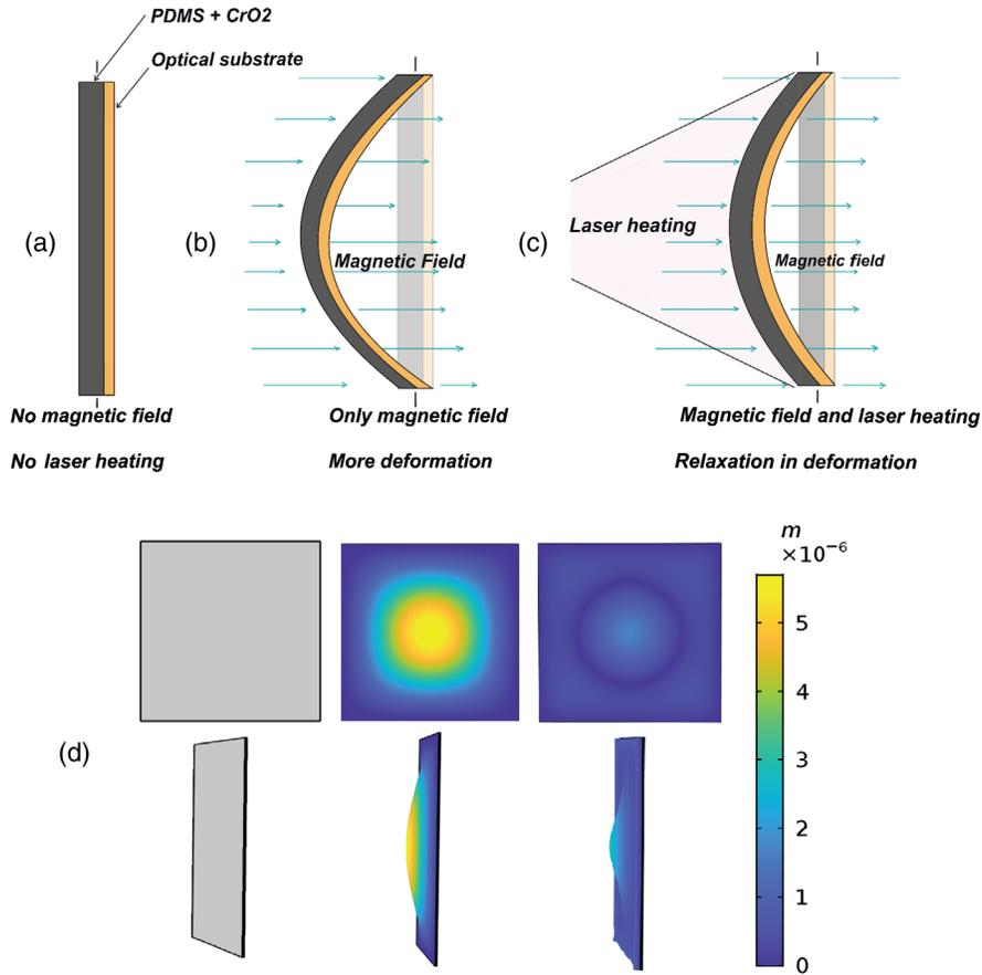
**Fig. 1** (a) Illustration showing the effects of (b) magnetic field and (c) laser heating on the PMADM. The magnetic field causes more deformation when the laser is off. The laser heats the PMADM surface causing demagnetization of the magnetic layer that results in relaxation. COMSOL simulation results of deformation at (d) Si-layer and cross-section view of the PMADM. All the edges of the PMADM are fixed.
