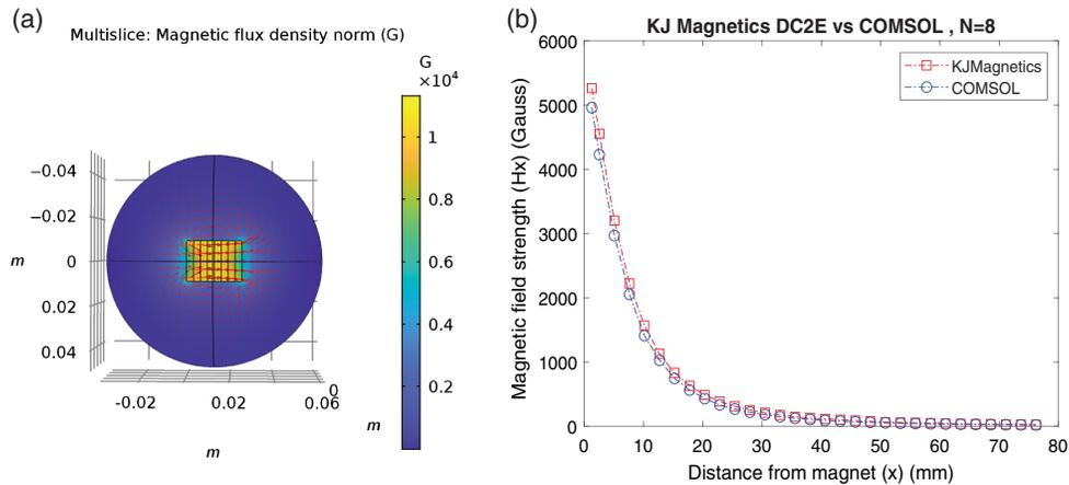
**Fig. 16** (a) Plot of magnetic flux density of eight KJ DC2E magnets in COMSOL. (b) Comparison plot of varying magnetic field strength with varying probe distance from the magnet. The RMSE percent error is 17%.
