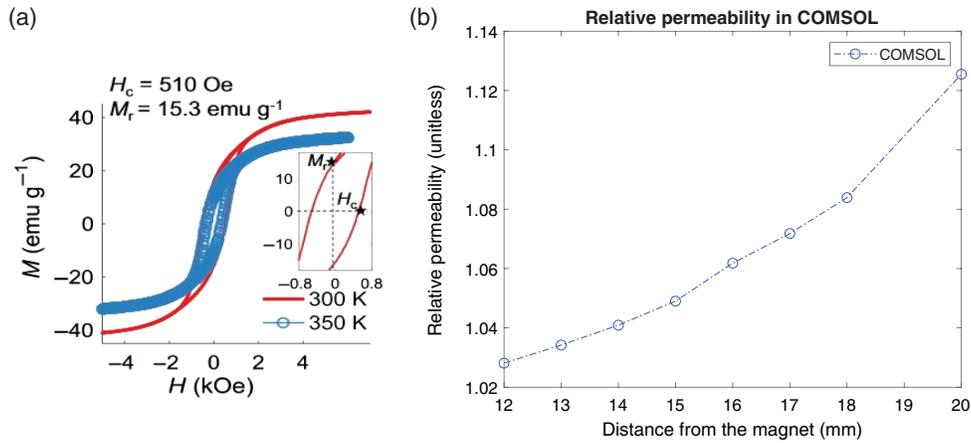
**Fig. 17** (a) Hysteretic plot of magnetization of CrO<sub>2</sub> by Li et al. (b) Plot of relative permeability with changing separation distance from the magnet.
