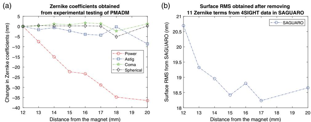
**Fig. 11** (a) Trend of Zernike coefficient terms obtained from experimental testing of the PMADM in the laboratory. A maximum change of 40 nm can be seen in the Zernike power terms when the separation between the magnet and the PMADM is increased from 12 to 18 mm. Other Zernike terms are stable to a maximum RMSE of 2.4 nm. (b) Surface RMS figure of the Si-layer of the PMADM is also shown. A maximum value of 21 nm is calculated, which makes our optical substrate functional as a mirror surface.
