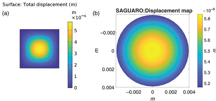
**Fig. 6** (a) Displacement due to the magnetic load on the Si-layer of the PMADM. (b) SAGUARO displacement map within the optical pupil diameter of the Si-side of the PMADM. A maximum displacement of  $5.7 \times 10^{-6}$  m is observed when the separation between the magnets and the PMADM sample is 12 mm.
