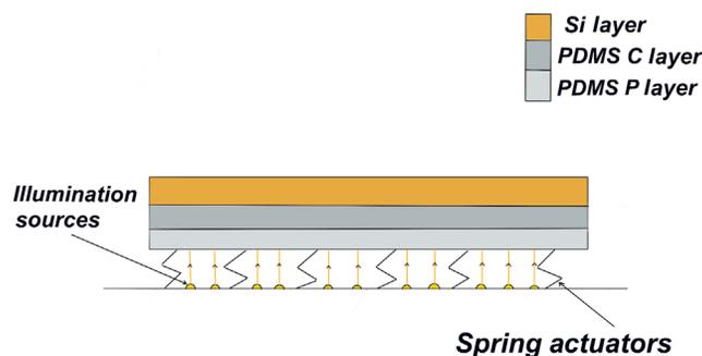
**Fig. 15** Illustration showing how the PMADM can be supported using spring actuators to facilitate scaling to larger areas. The magnetic load will compress the springs and will help in keeping the mirrors flat. Local demagnetization will allow relaxation of springs locally providing more spatial control. Demagnetization of the magnetic layer can be achieved using illumination sources as shown in the illustration.
