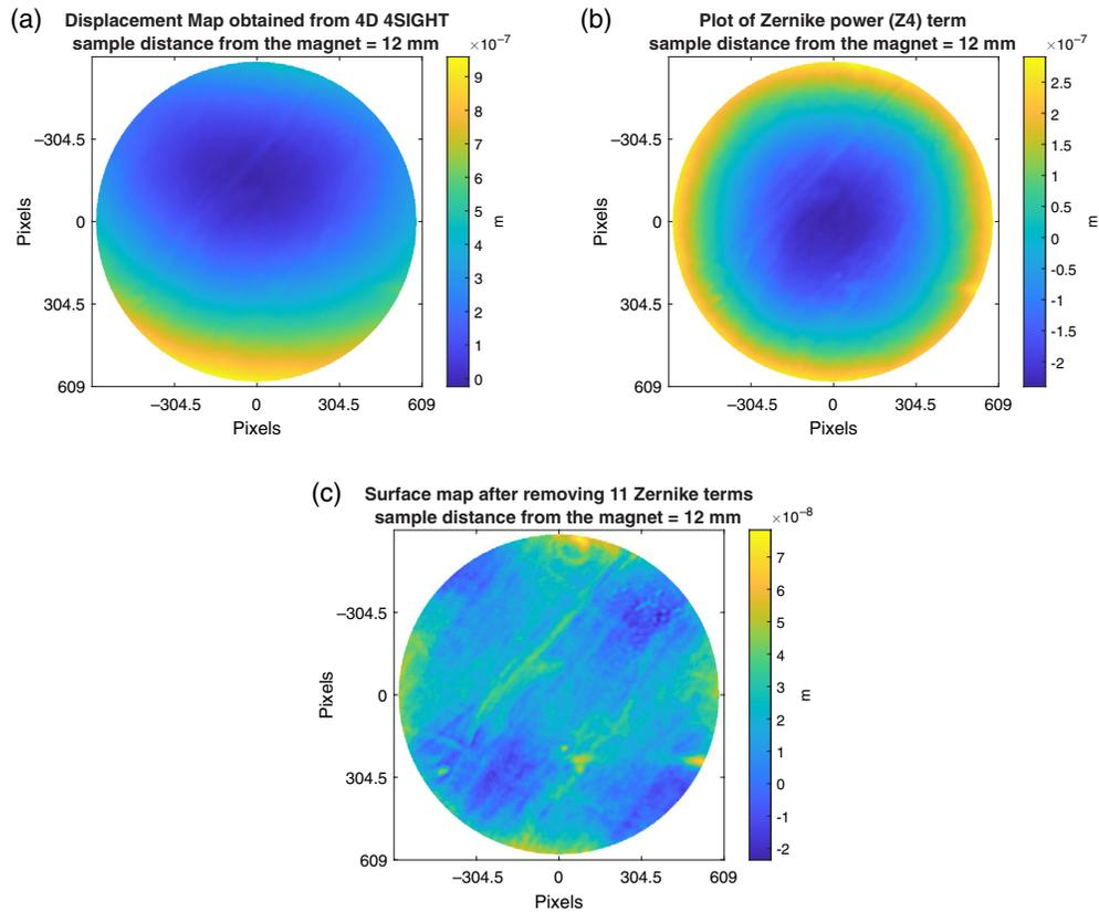
**Fig. 10** (a) Displacement map obtained from experimental testing of the Si-layer of the PMADM sample using a 4D interferometer<sup>51</sup> when the sample is 12 mm from the magnet. (b) Zernike power terms obtained after postprocessing the displacement map in SAGUARO. (c) To quantify the residual roughness, a map after subtracting 11 Zernike terms is shown with surface RMS of  $\sim 21$  nm. Residual mounting stress is seen through a four-sided pattern.
