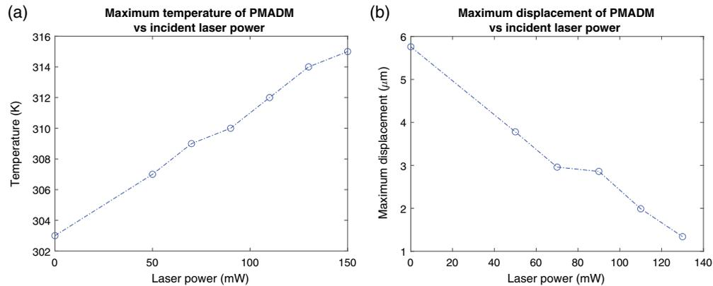
**Fig. 9** (a) Simulated PMADM temperature (measured at the P-layer) with varying laser power. (b) Maximum displacement due to both magnetic loading and laser heating at the Si-layer of the PMADM at different incident laser powers. As the laser power increases, more heating causes a temperature increase, which in turn, causes a decrease in magnetization and magnetic loading that results in more relaxation.
