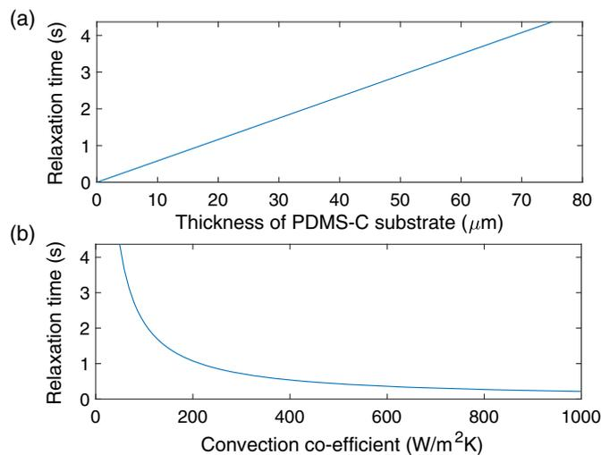
**Fig. 18** Simulation of relaxation time of PMADM for (a) different thicknesses of PDMS-C layer and (b) heat convection coefficient. The relaxation time can be improved linearly by reducing the thickness of the PDMS-C layer or can be improved exponentially by increasing the heat convection coefficient.
