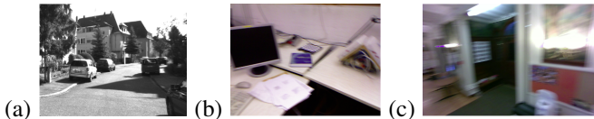
Fig. 2: Typical turning sequences from vehicle-mounted (a), hand-held (b), and head-mounted (c) cameras demonstrate the potential for comparatively severe blur in head-mounted sequences.
