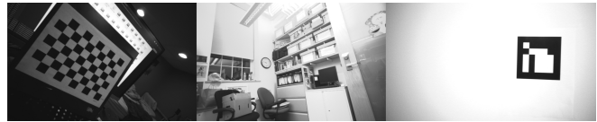
Fig. 4: Left to right: A sample checker board image, an image in the sweep exposure set, and a sample vignette image used for calibration.
