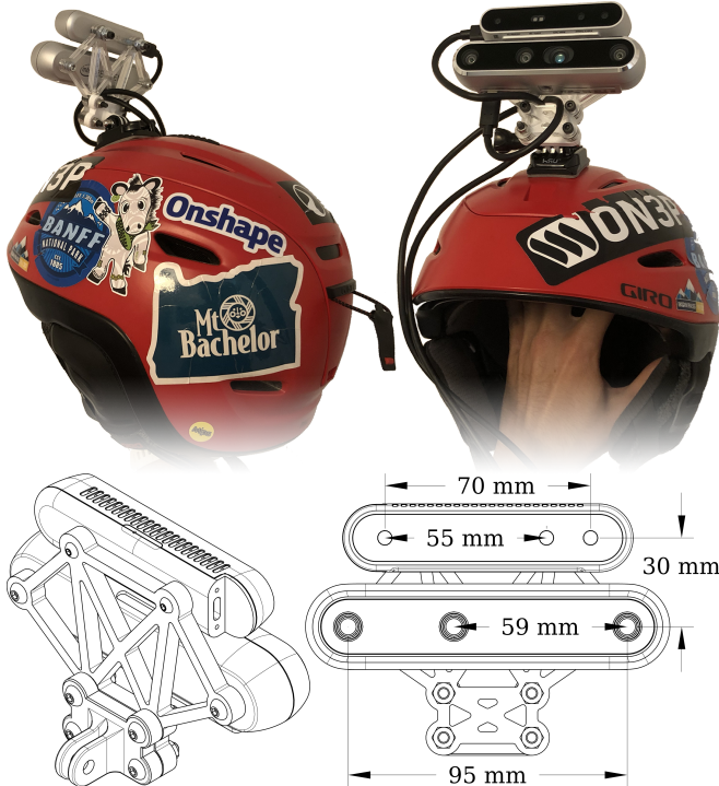
Fig. 3: Two views of the camera assembly, shown together with frontal inter-camera measurements and CAD drawings.
