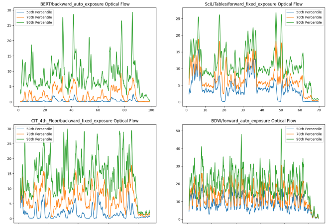
Fig. 11: Plots of optical flow magnitude across our sequences show that BPOD is characterized by sudden, rapid movements that produce spikes in optical flow.
